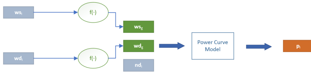
Figure 20. “Ideal” power curve model based on the free stream wind speed wsg , the free stream direction wdg and the yaw misalignment nd_i of each WTG.
