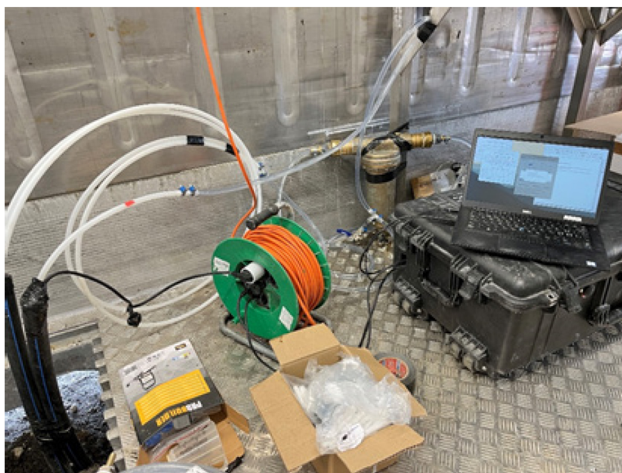
Figure 17: The miniRUEDI is continuously running inside the CARBFIX container. The black suitcase is the miniRUEDI, and the computer serves as a screen displaying real-time monitoring results.
