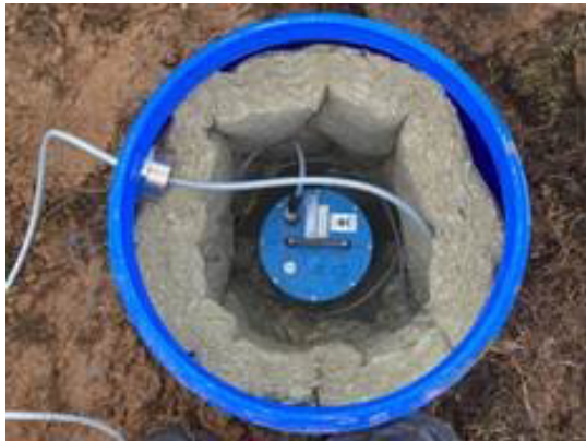
Figure A3: Sensor with thermal insulation installed.
