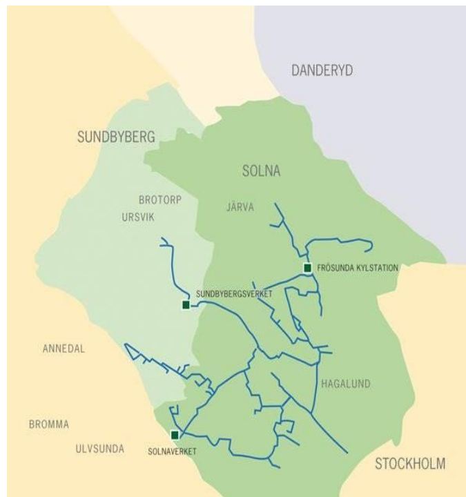
Figure 11: DC system of Norrenergi AB – the three cold production plants Sundbybergsverket, Frösundaverket (kylstation) and Solnaverket (where the existing cold storage is also located)
