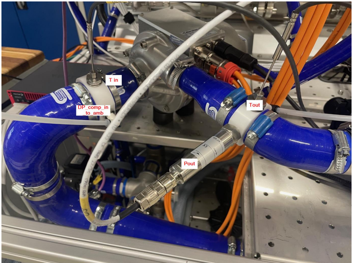
Figure 20: Validation on OPmobility fuel cell test bench – building block compressor 1 prototype installation and sensor positions.
