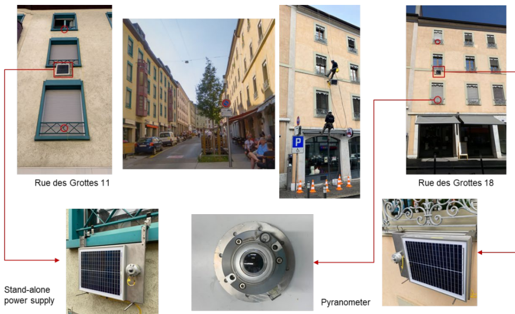
Figure 7. Solar radiation monitoring station on an urban canyon in Geneva (rue des Grottes).
