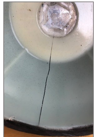
Figure 10: Complete liner assembled by welding (left) and crack appearing in the liner around the metal insert because of the high thermal shrinkage of polymer A
