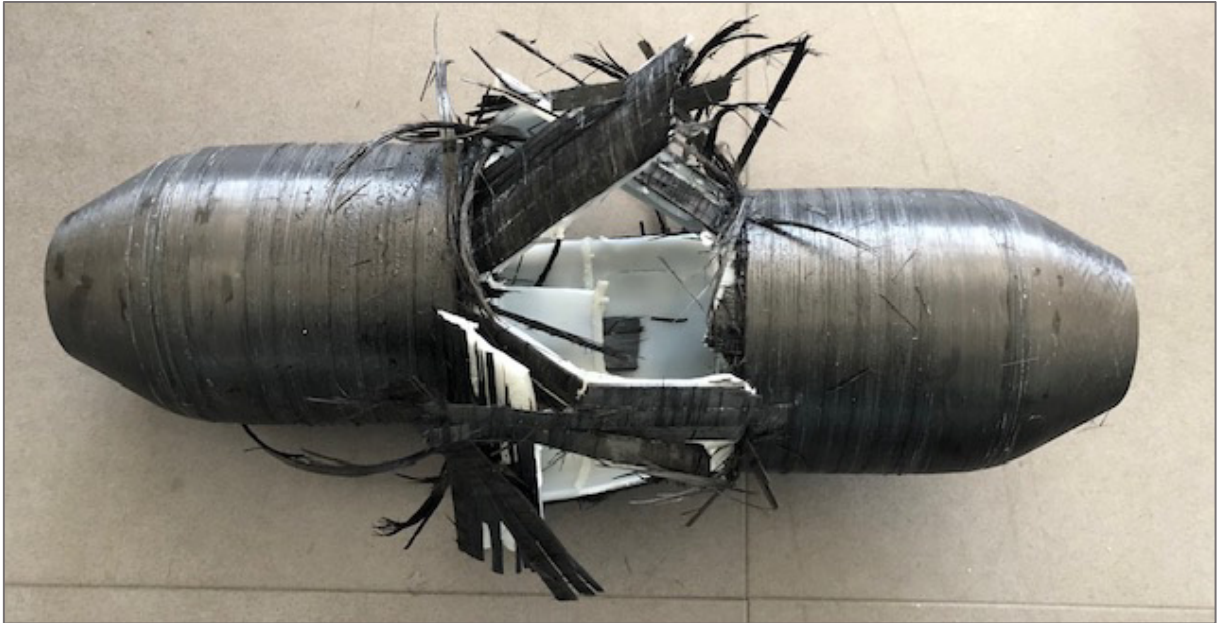
Figure 15: Pressure tank prototype after burst
