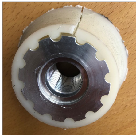
Figure 10: Complete liner assembled by welding (left) and crack appearing in the liner around the metal insert because of the high thermal shrinkage of polymer A
