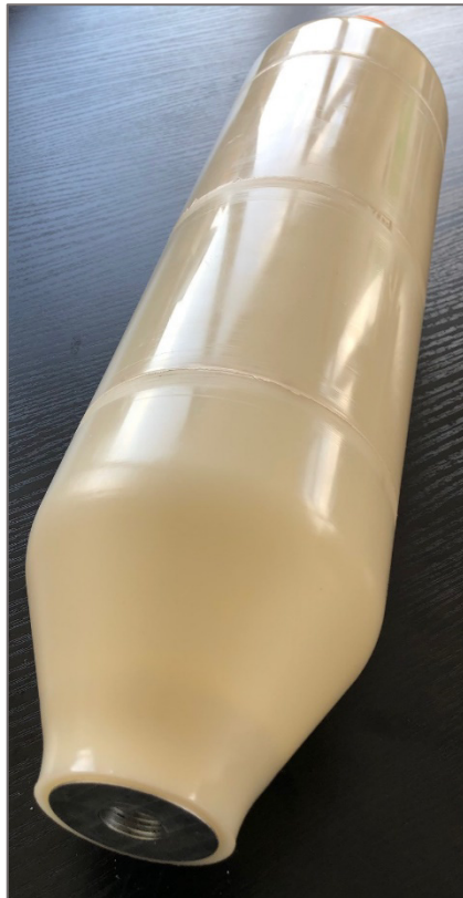
Figure 10: Complete liner assembled by welding (left) and crack appearing in the liner around the metal insert because of the high thermal shrinkage of polymer A
