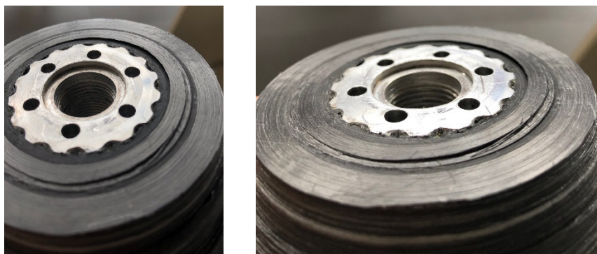
Figure 15: Extrusion of the first layer at 90°.
