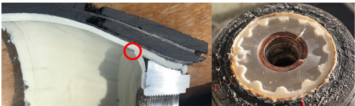
Figure 12: tank failure due to the extrusion of the liner
