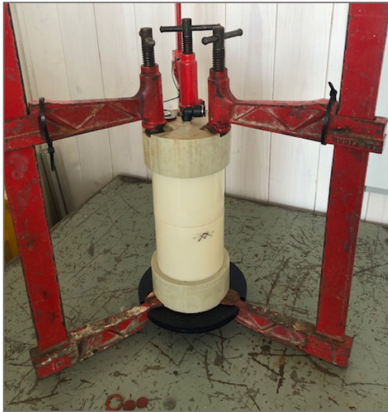
Water tightness test setup developed to evaluate the performance of welding assembly
