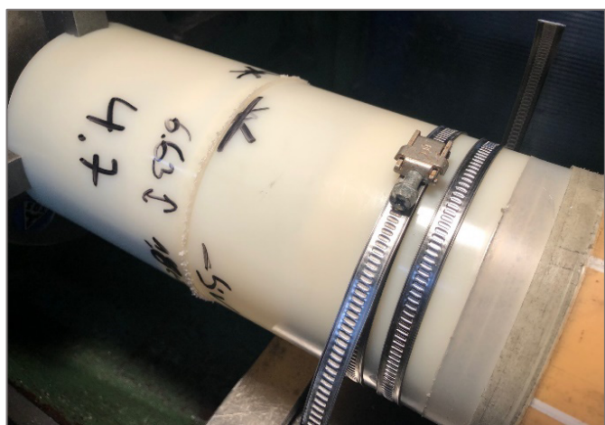
Figure 8: L, Z, V welding profiles (top) and fixtures developed to hold the part, machine the welding profiles and perform spin welding
