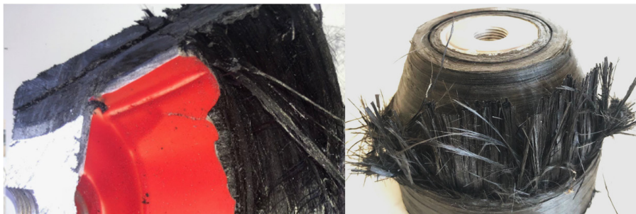
Figure 10: burst test; the Polymer A-CF prototype burst at 550 bar
