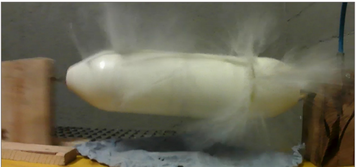
Figure 14: Burst test of a liner
