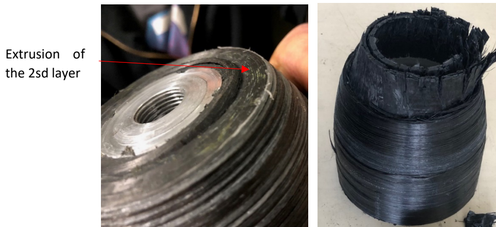
Figure 16 : Extrusion issue observed at 1206 bar and bust of the tank appeared at 1235 bar
