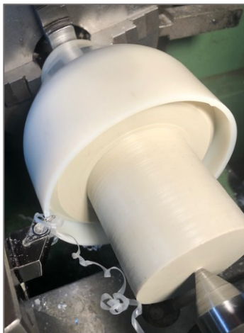
Figure 8: L, Z, V welding profiles (top) and fixtures developed to hold the part, machine the welding profiles and perform spin welding
