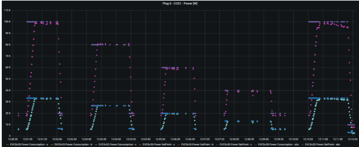
Figure 20: Results of GoFast station controllability experiment: Active power setpoint vs. implementation
