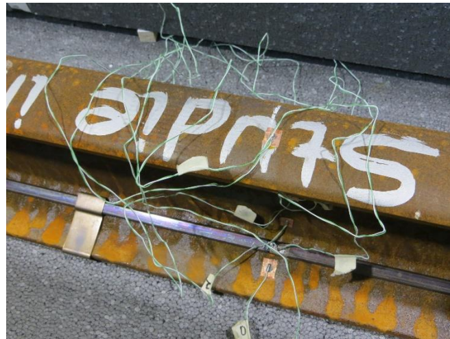
Figure 11: glued copper lamellas with thermocouples on top
