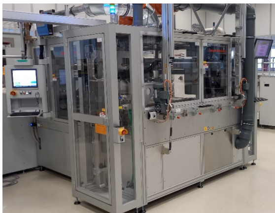
Figure 8: Picture of the new installed PECVD automation from J&R company and sketch of the new PECVD system for the tunnel junction deposition
