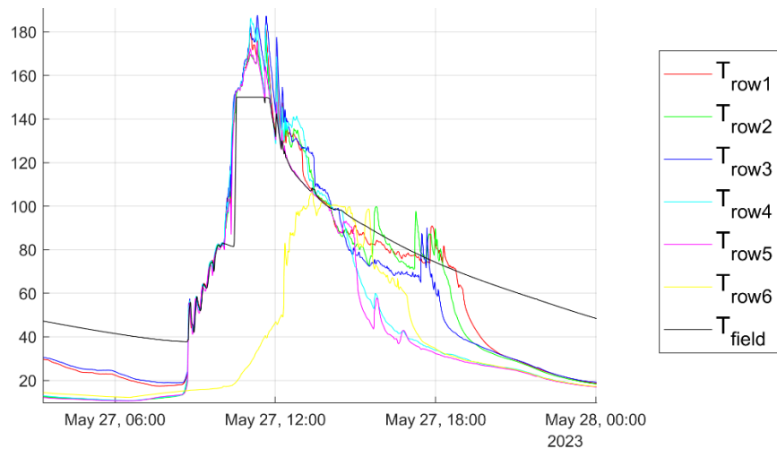
Figure 8: Collector row temperatures measured on the 27.5.2023. The peak temperature reached 187.73 °C \pm 0.52 °C in row 3. The horizontal line of T_{\text{field}} between 11 and 12 a.m. is assumed to be a display cut-off.
