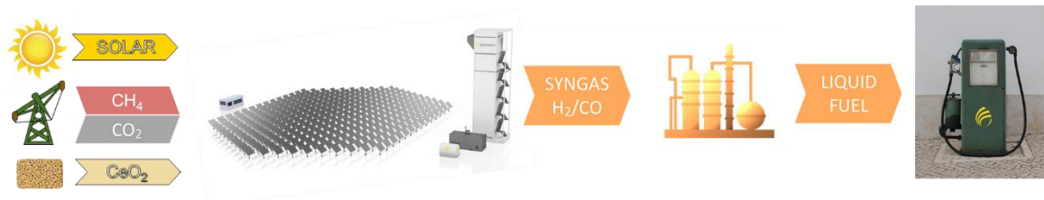
Figure 1: Dry redox reforming process to produce drop-in liquid fuels
