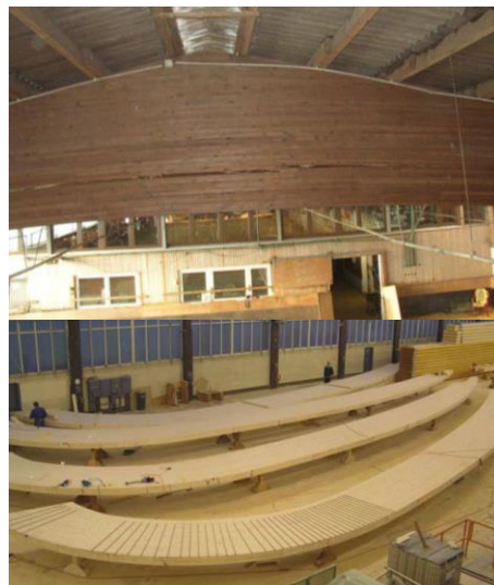
Figure 2: Transverse tensile failure of a pitched roof girder (top), production of curved beams with reinforcements by threaded rods (bottom), Brüninghoff (2007)
