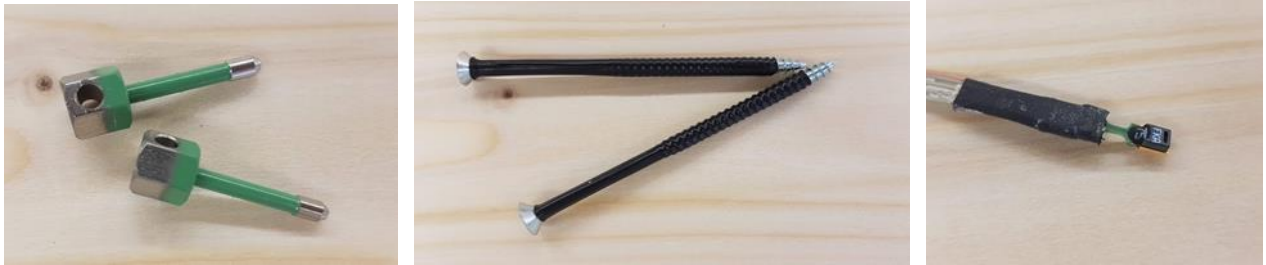
Figure 14: Partially Teflon coated GANN electrodes (left), partially insulated screws (middle) and CMOS relative humidity and temperature sensor (right).
