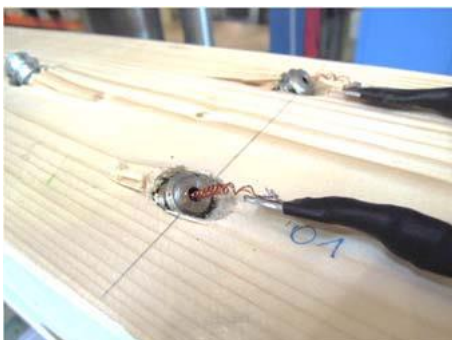
Figure 5: Strain gauges inside the reinforcement, source: Dröscher (2016)
