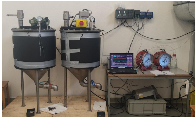
Figure 4: Tandem digesters set-up
