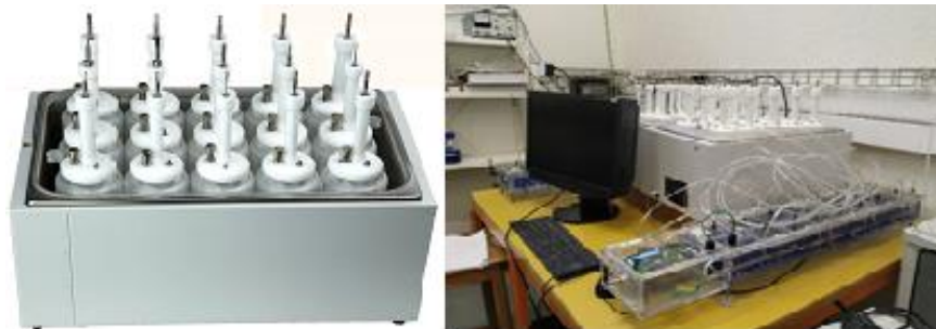
Figure 7: Biomethane potential (BMP) reactors set-up
