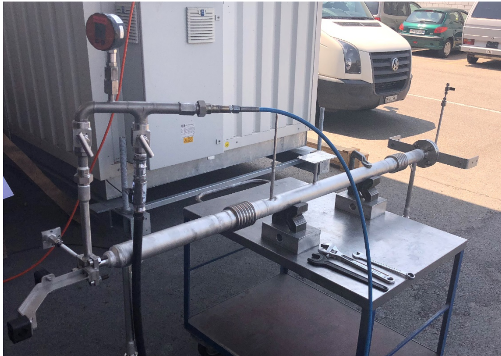
Figure 7: Polytopic Methanation Reactor R-51 during factory acceptance test for pressure.
