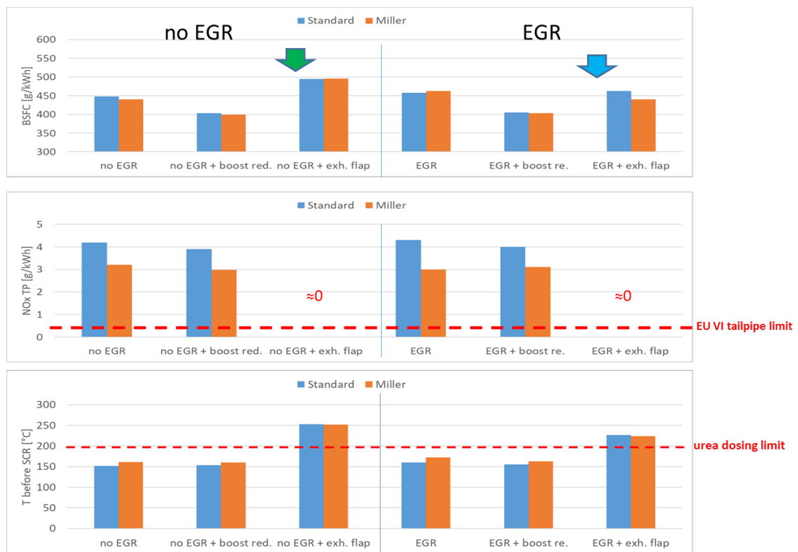
Figure 31: Summary of temperature and NO x management measures for engine out NO x target of 5 g/kWh at low load operation point 1050rpm/230Nm
