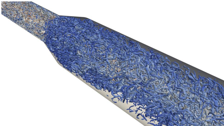
Figure 41 - Turbulent structures in conical diffuser
