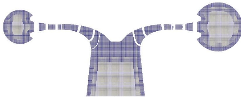
Figure 78 - Pump-turbine mesh, side view, grid A
