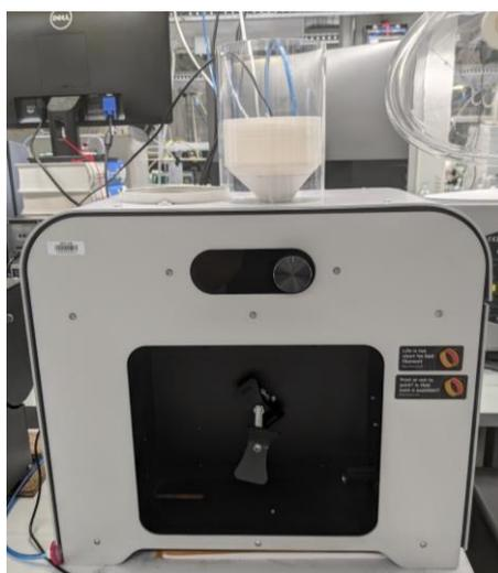
Figure 1 - Composer 450 (3Devo, Netherlands) used for the extrusion of biocomposites.
