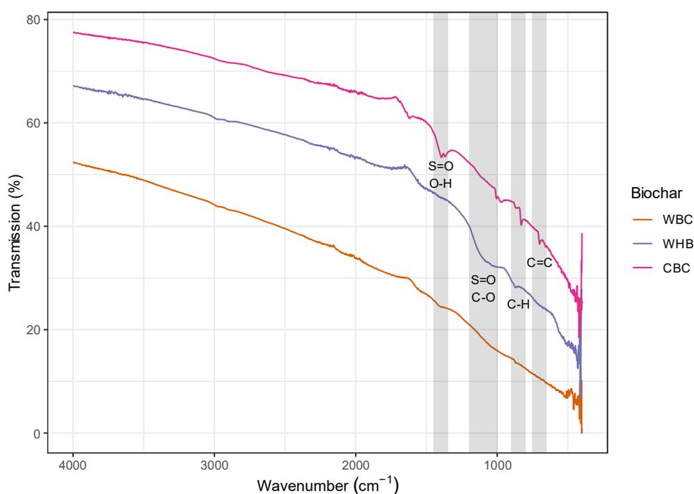
**Figure 8** - FTIR spectra for three biochars. Peaks are labelled.
