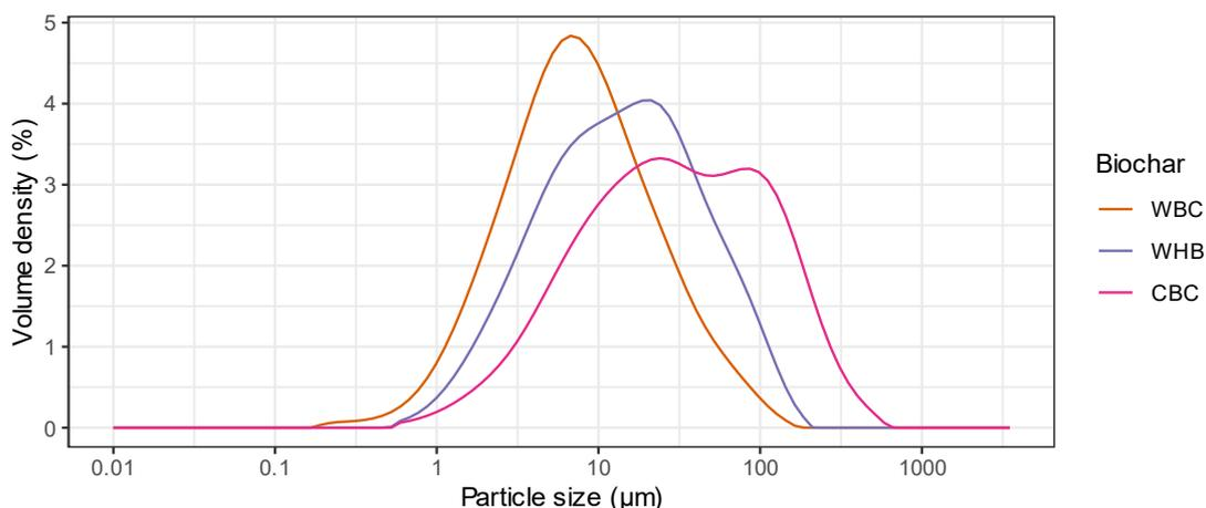
**Figure 6** - Particle size distribution for biochars. Values based on an average from 6 replicate measurements.
