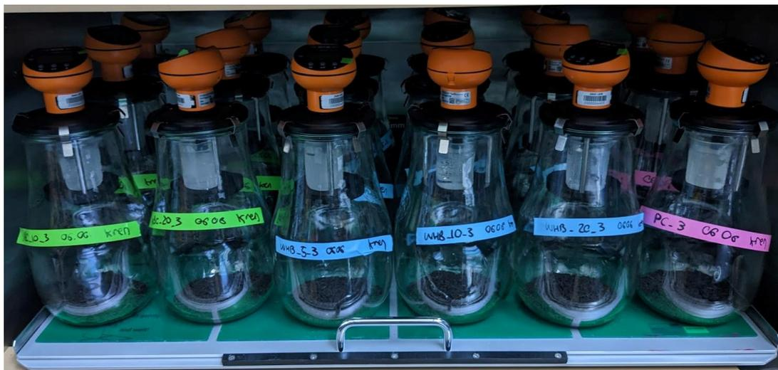
Figure 2 - Biodegradation experiments performed in an incubator at 58 °C.
