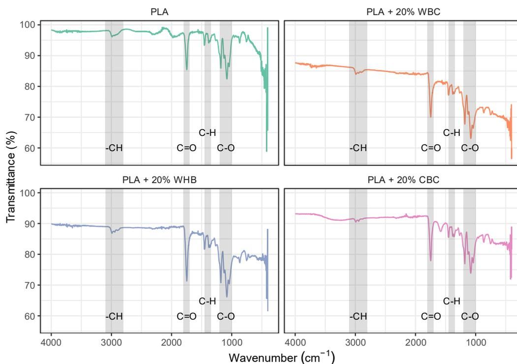
Figure 12 - FTIR spectra for pure PLA and biocomposites containing PLA and 20 wt. % biochar.
