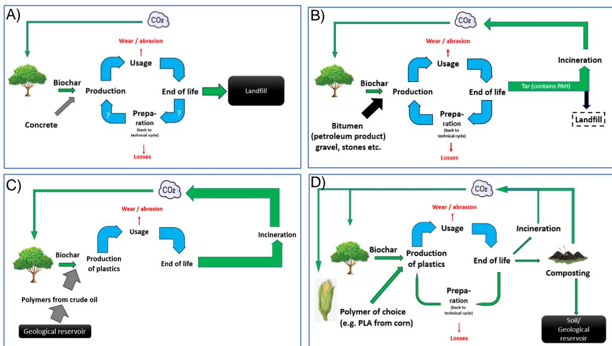
**Figure 5** - Four use cases for C-sequestration using biochar in a circular context. A) Addition of biochar to concrete; B) Addition of biochar to asphalt; C) Addition of biochar to plastic polymers from fossil sources, without recycling; D) Addition of biochar to plastics polymer from renewable sources, with biochar recycling
