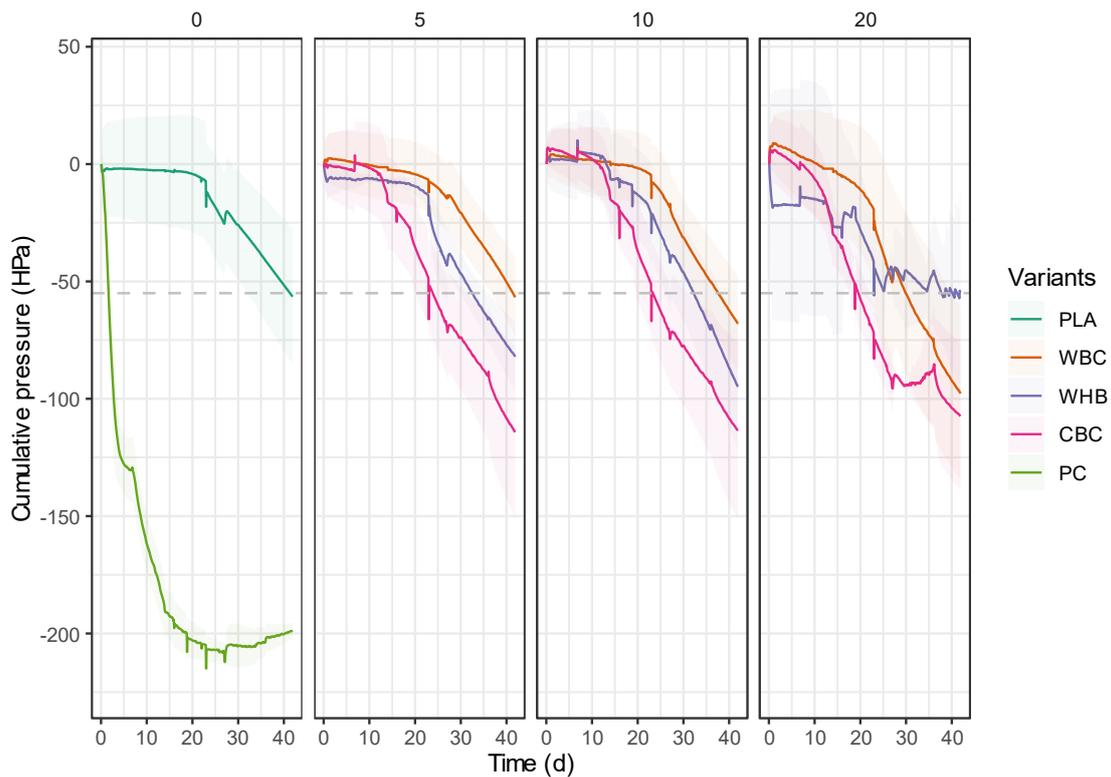
**Figure 13** – Preliminary mean ( $n = 2$  for 20 wt. % variants and  $n = 3$  for others) biodegradation results within the first 40 days of degradation. The plot on the left contains variants without biochar such as PLA and a rapidly degradable positive control (PC). The plot in the middle and on the right show the consumption of oxygen during the degradation of biocomposites containing 5, 10 and 20 wt. % biochar. The shaded area represents the standard deviation.
