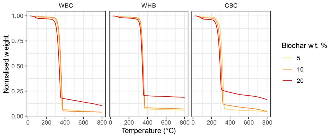
**Figure 15** – Thermal degradation of biocomposites arranged by added biochar weight.
