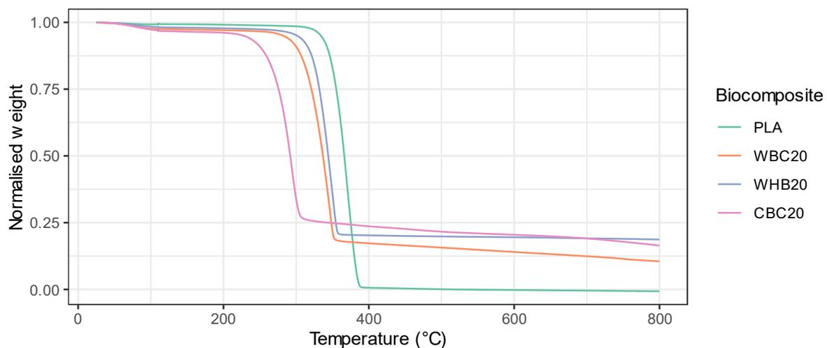
**Figure 14** - Thermal degradation of pure PLA and biocomposites consisting of PLA and 20 wt. % biochar under oxygen free conditions.
