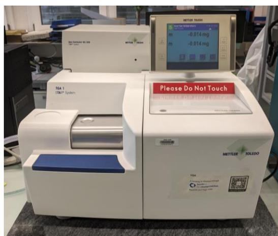
Figure 3 - Thermogravimetric Analysis Device used for measurements.
