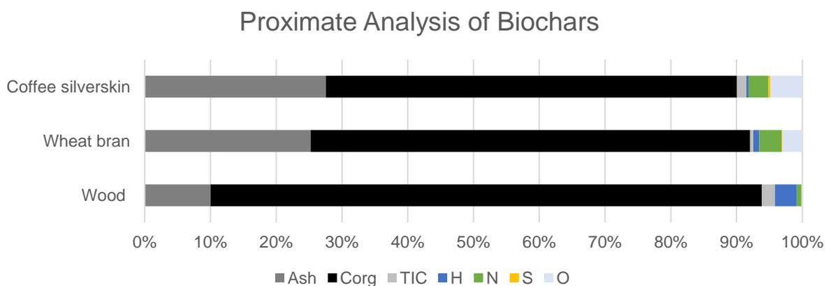
**Figure 7** - Proximate analysis of biochar produced from coffee silverskin, wheat bran and wood. Data from Gutzwiller et al., (2022)
