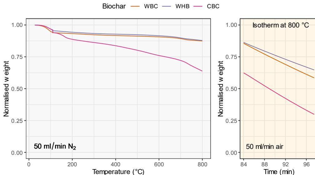
**Figure 9** - Thermal degradation of biochars under inert conditions between 25 - 800 °C (left) with an additional isotherm performed under atmospheric conditions at 800 °C for 15 minutes.
