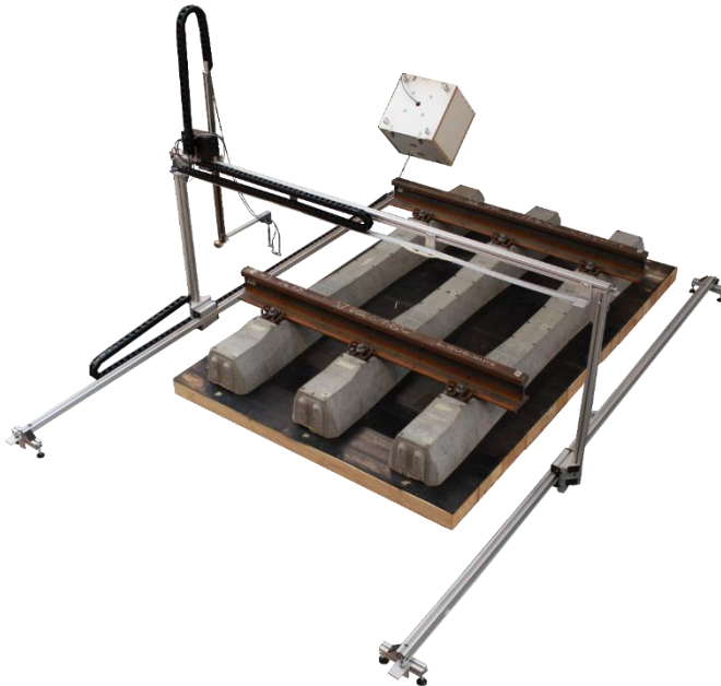
Figure 23 – The three-sleeper cell, with the automated gantry used for acoustic measurements, and the electromagnetic shaker set-up for a 45° excitation.
