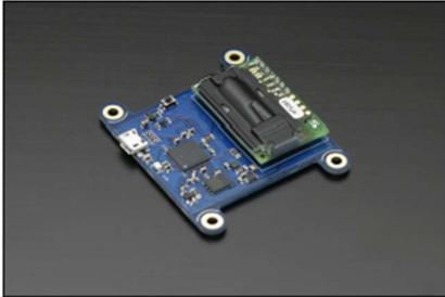
The Yocto-CO2-V2 device lets you measure the quantity of carbon dioxide (CO<sub>2</sub>) in ambient air as well as the relative humidity, temperature and atmospheric pressure via an USB connection. It can record the measurements on its internal flash for later retrieval when connected again by USB.
