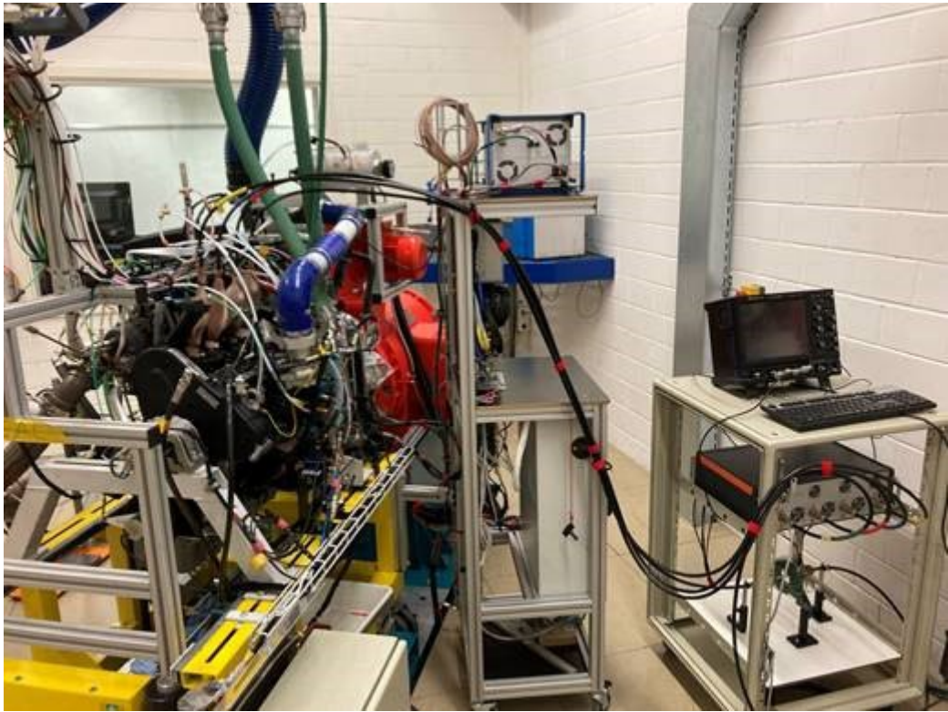
Figure 6: Engine setup with 4-channel pulse generator for NRPD ignition.
