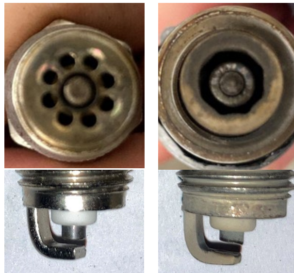
Figure 54: Sparkplug wear under NRPD ignition for surface discharge sparkplug (top) and j-type electrode (bottom)
