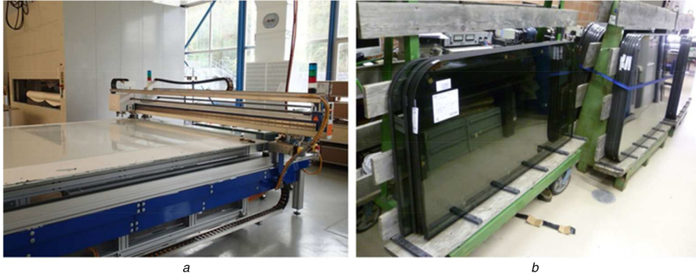
Fig. 3 To produce real size windows a computer numerical control CNC table with a large working dimension of 2.5 \times 3 \text{ m}^2 was equipped with a laser engraving system (Nd YAG laser) and a series of 34 windows of 1 \times 1.4 \text{ m}^2 was produced
