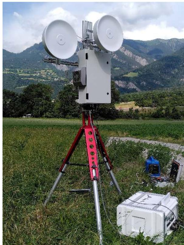
Figure 4.4: Image of the radar target simulator (RTS). The radar pulses are received by the round antenna on the right. The modulated and delayed pulses are sent back towards the radar by the antenna on the left.
