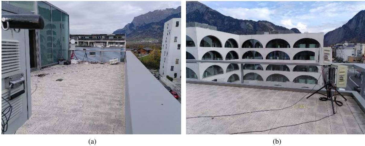
Figure 4.8: Set-up of the wind park simulation experiment on the roof of our office building in November 2022. (a) Radar receiver in the foreground, target simulator and transmitter in the background. (b) Image of the radar receiver.
