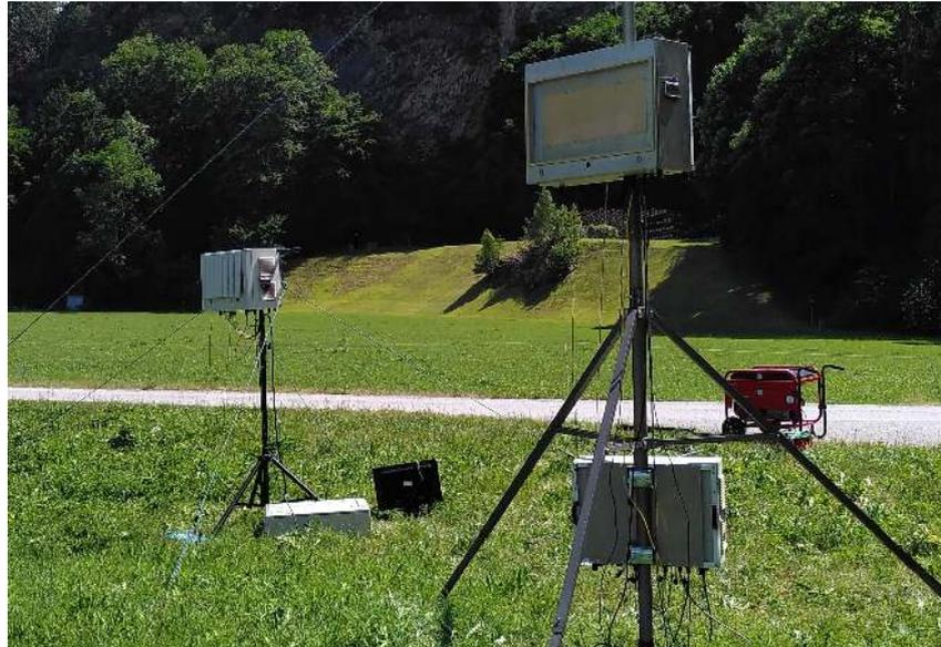
Figure 4.3: Bi-static C-band radar used for the measurements. The transmitter is on the right and the receiver on the left.
