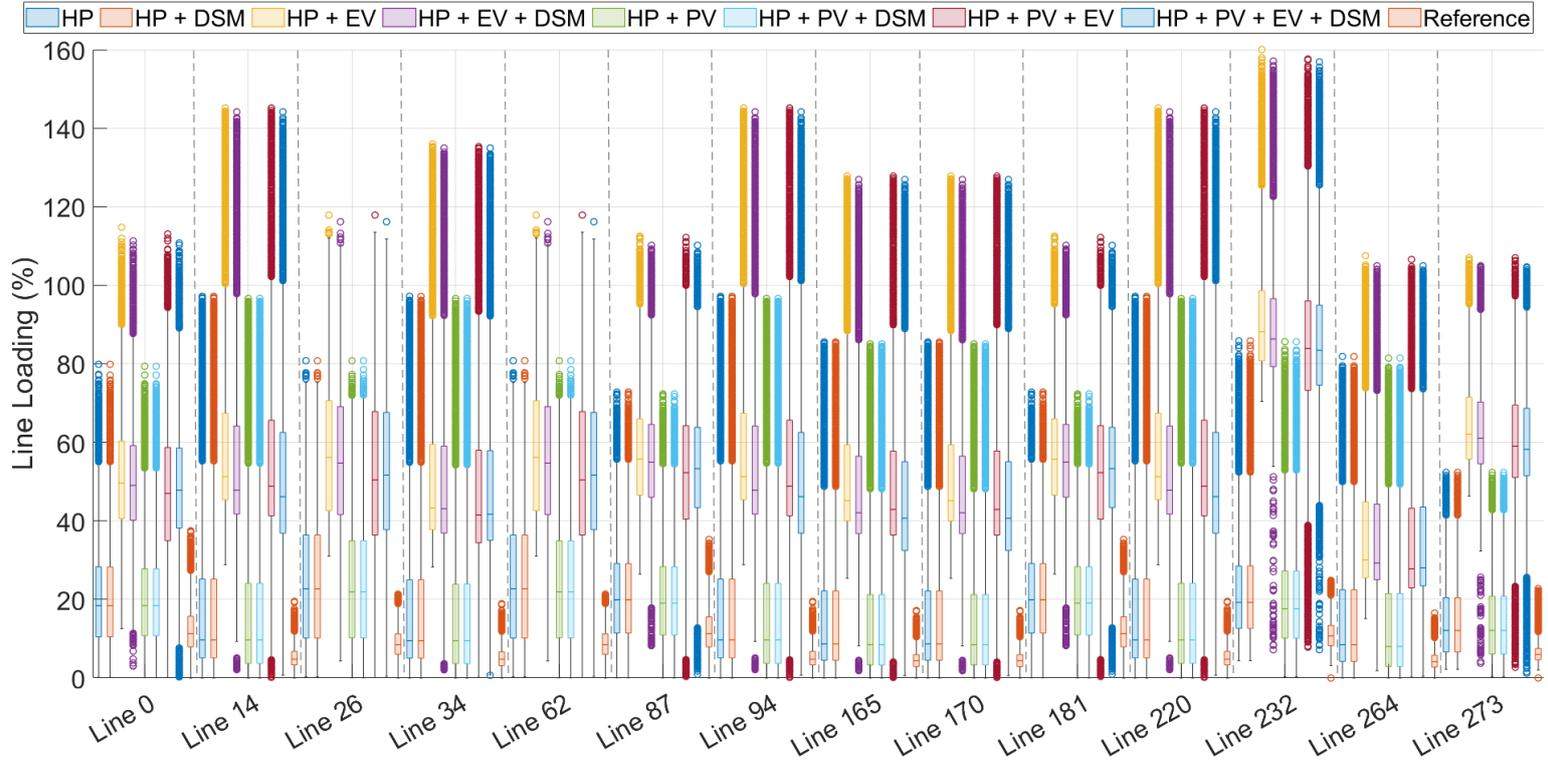
**Figure 23: Most loaded lines of TS 1 grid for the scenario with additional 73 HP, 99 EVSE and 51 PV.**
