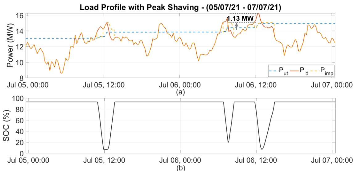
**Figure 18: Results applying the proposed control scheme: (a) Total load curve of Arbon city and imported power from the grid, and (b) SoC of BESS.**
