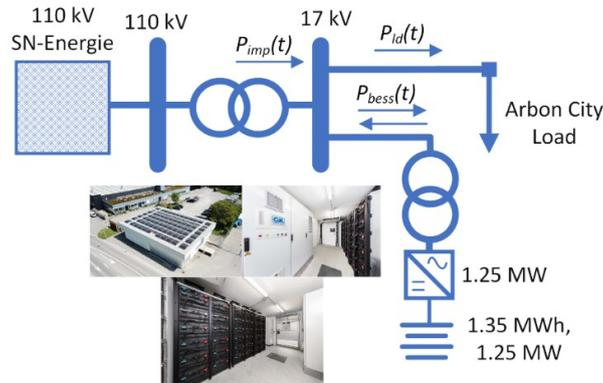
Figure 1: Simplified schematic of the entire system.
