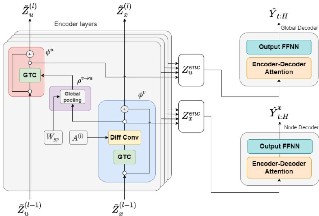
Figure 10: GNN with global attribute and pooling from nodes towards global [12].
