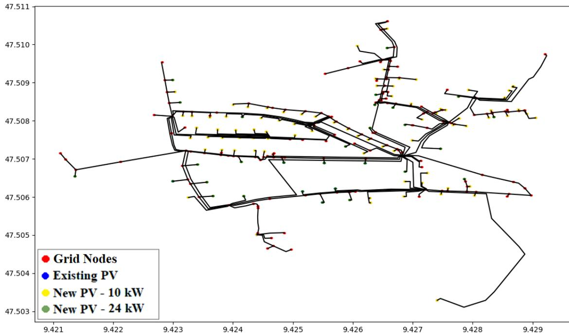
Figure 2: LV distribution network supplied by TS 1 – Scenario with 111 new PV
