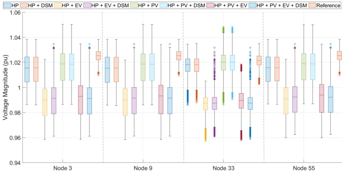
**Figure 21: Most loaded nodes of TS15 grid for the cases of the worst-case scenario.**
