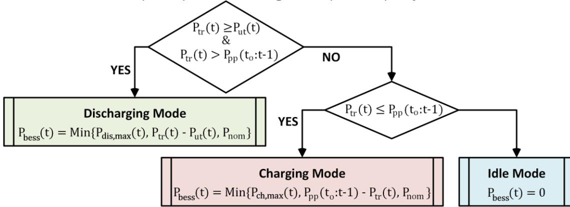
**Figure 12: Logic diagram for the determination of each BESS mode.**
