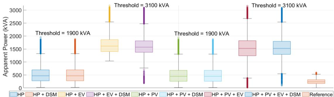
**Figure 24: Apparent power of TS 1 transformer for the cases of the worst-case scenario.**
