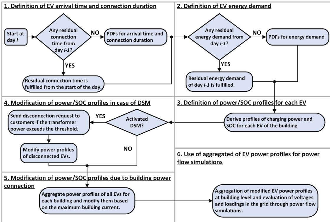
**Figure 13: Procedure followed for the generation of total EV power profile in each building.**
