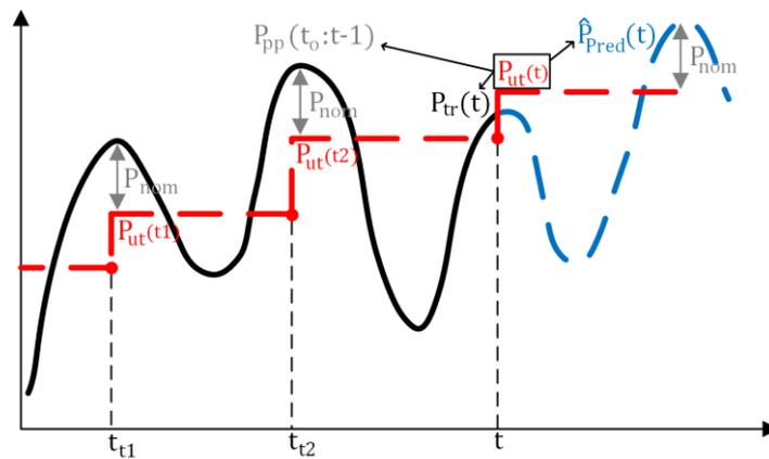
Figure 11: Concept for the update of threshold used for BESS charging and discharging.
