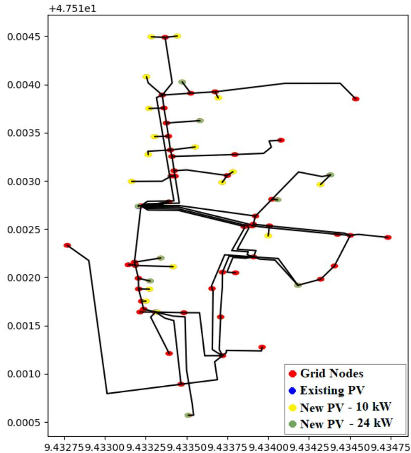
**Figure 3: LV distribution network supplied by TS 15 – Scenario with 27 new PV**
