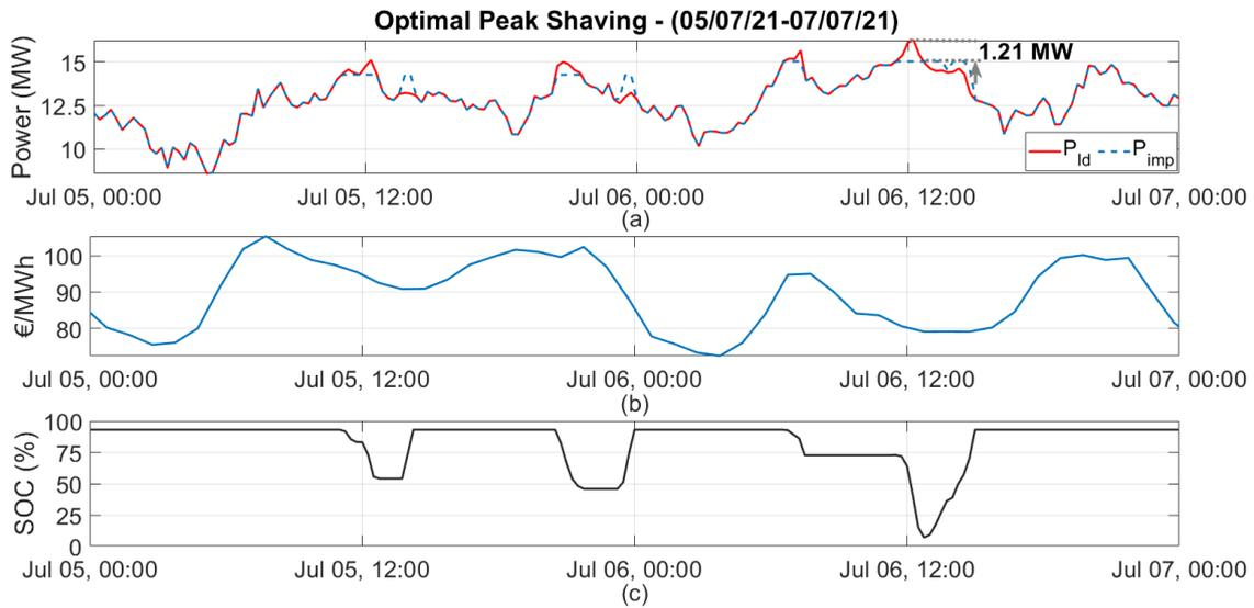
**Figure 17: Results applying the optimization-based approach: (a) Measured power load vs. power load with BESS operation, (b) EPEX Spot price, and (c) SoC of BESS.**
