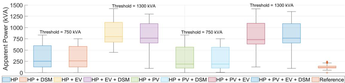
**Figure 20: Apparent power of TS 15 grid for the cases of the worst-case scenario.**
