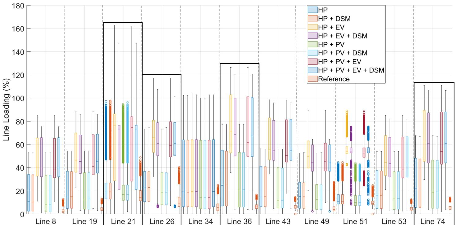
Figure 19: Most loaded lines of TS 15 grid for scenarios with 27 new HP, 27 new EVSE and 27 new PV.
