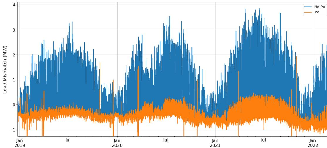
**Figure 4 Mismatch between the aggregate load of all smart meters and the load measured at the MV transformer due to inconsistencies in measurements.**
