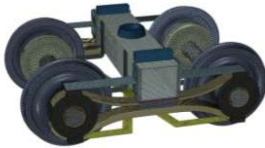
Figure 17- Finite element model (Mesh view) of the FRP bogie
