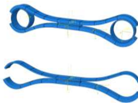
Figure 15- Simplified 3D models of the FRP bogie
