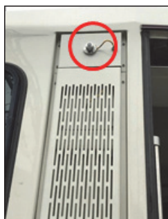
Fig. 8: Solar radiation sensor (1 of 2)
