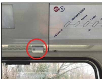
Fig. 6: Temperature / humidity sensor (1 of 8)
