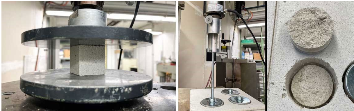
Figure 35. Left: Picture of the compressive strength test. Right: Picture of the pull-out test.
