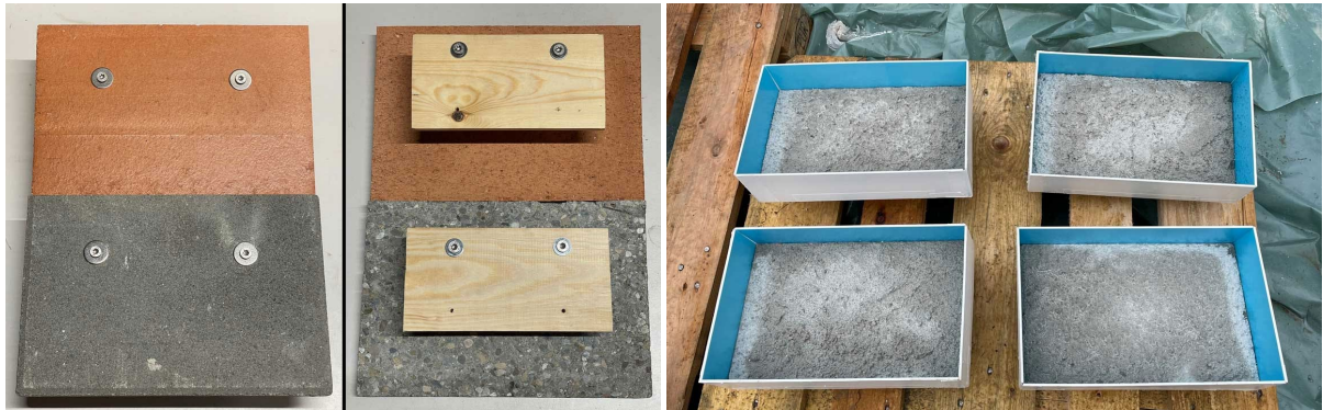
Figure 32. Testing plates (brick and porous concrete). Left: Plates with hanging setup. Right: Plates with pre-spraying mortar and coating applied as well support for the application of 6 cm of insulating render.
