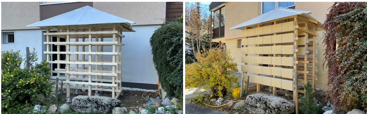
Figure 34. Left: Wooden structure built for the testing plates. Right: Testing plates placed in the wooden structure.
