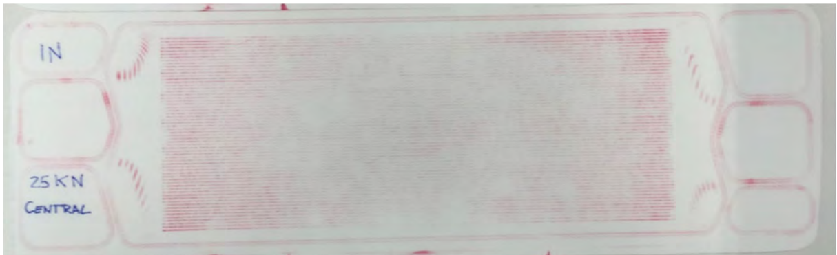
Figure 26: Visualization of compression force with pressure sensitive film
