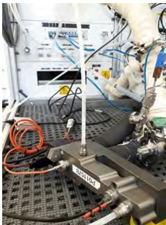
Figure 33: Test setup for ejector / valve combination and CFD simulation of ejector
