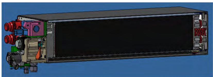
Figure 10: The housing is completely closed on the back side of the FC. A bus bar brings the plus pole to the front side junction box
