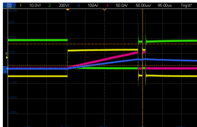
Figure 9. Typical switching waveforms for the XS-cross hybrid switches (yellow- gate source voltage, green- voltage across device, pink- current through device, blue-inductor current)
