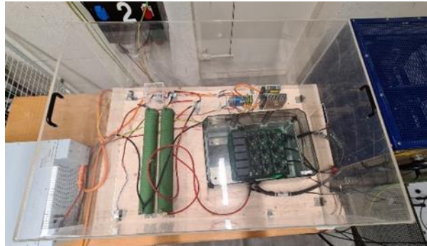
Figure 17. Converter hardware Inside Protection Cage
