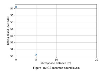
The first set of tests unveiled that the UAV noise emissions were always inside the NAO specifications. In one case (UAV take-off) the result was over the threshold because of the microphone was placed right below the taking-off UAV, an unrealistic position for a person in normal operations.
