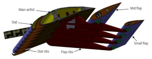
Figure 40 Modified SP180 main wing design
