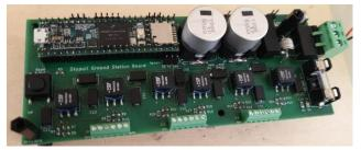
Figure 71: Teensy 3.6 Control Board
