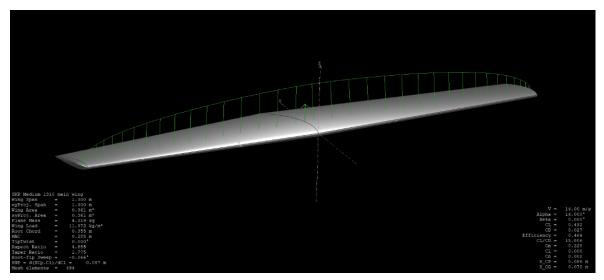
Figure 24: Load Distribution in the Main Wing
