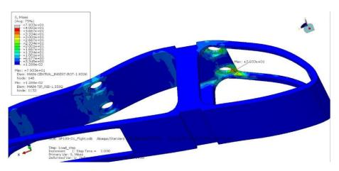
Figure 41 FEM analysis on Mises stress on central insert of lower main wing
