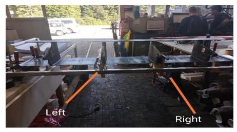
Figure 45: Static test on the main wing of SP130-03
