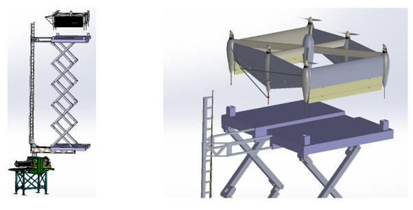
Figure 65: Study of a Ground Station with take-off /landing platform
