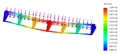
Figure 39 Maximum Displacement for loading conditions
