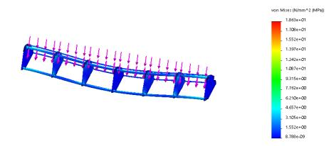
Figure 38: SP 180- 01 Main Wing Von Mises Stress distribution for loading conditions
