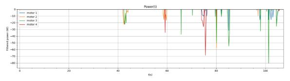
Figure 16: VESC power consumption plot (negative values represent power generation)
