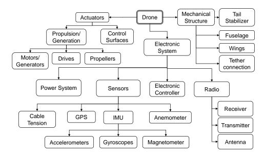
Figure 80: Drone structure considered for the FMECA
