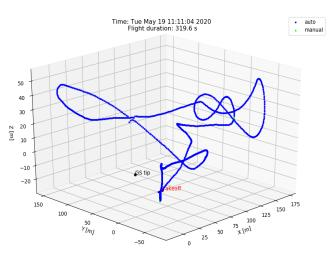
Figure 20: UAV trajectory during fully autonomous flight
