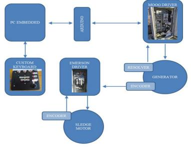
Figure 62: Ground Generation System Scheme
