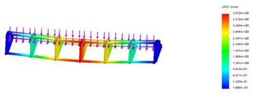
Figure 33: Maximum Displacement for loading condition
