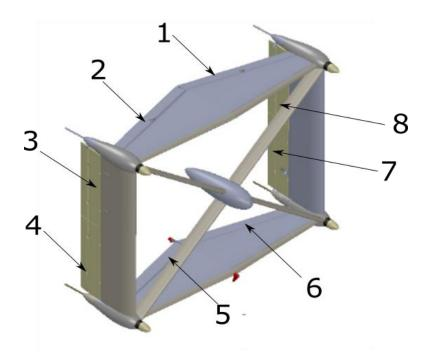
Figure 26: Flight Control Surfaces of SP130-02
