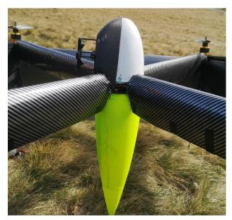
Figure 53: UAV ultrasonic wind sensor implemented
