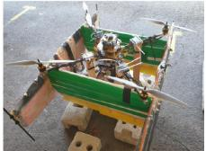
Figure 75: Bench test of a UAV used to test electronic components
