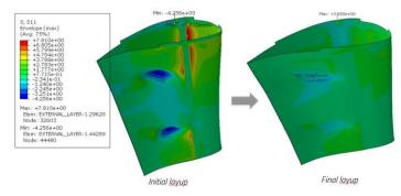
Figure 42 Study on reduction of stresses on external fibres layers on the SP180 main wing due a new layup
