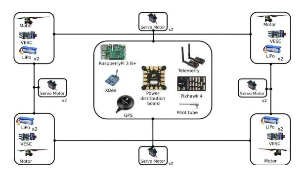
Figure 48: System Architecture
