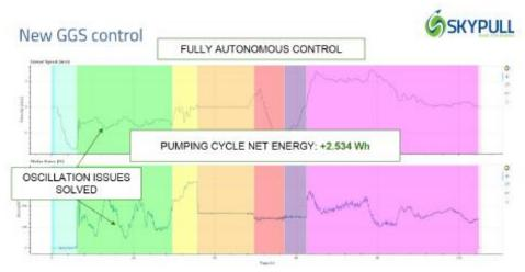
Figure 68: Result obtained by using the new GS control strategy
