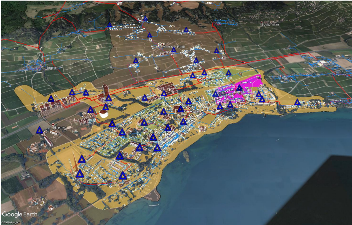
Figure 3: Transformer in the RE Demo zone (triangles) with TR3716 within the references case area (magenta).
