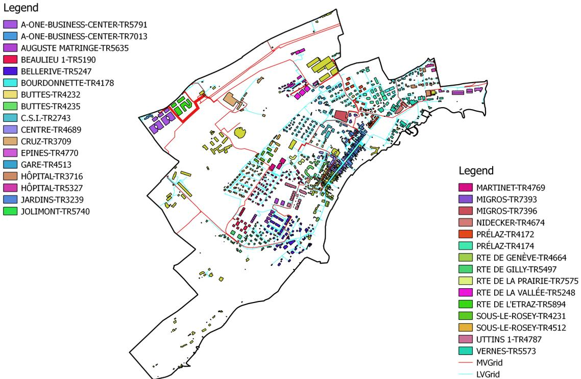
Figure 4: Localization of buildings unit elements according to their LV transformer
