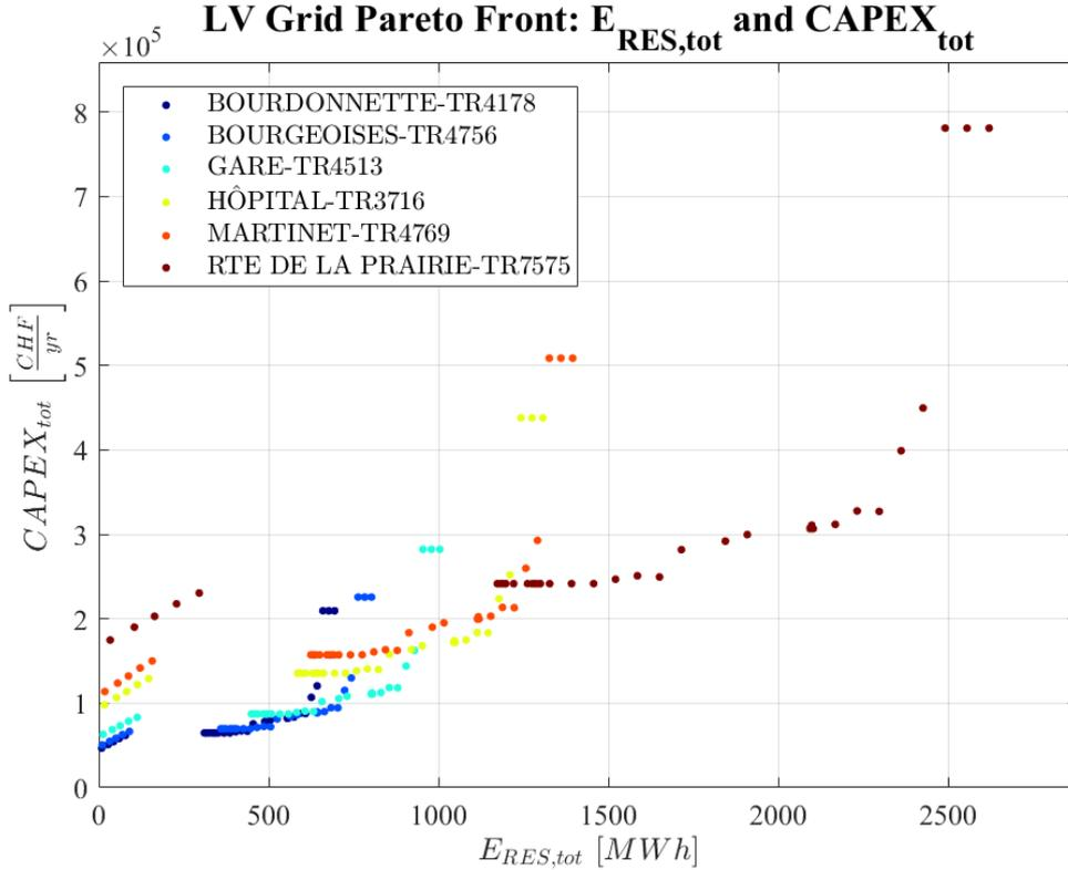
Figure 14: Aggregated Pareto curves for the 6 preselected LV grids
