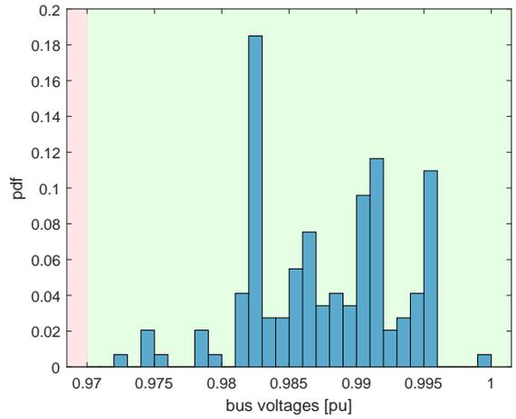
Figure 16: Normalized histogram of the bus voltages without any generation
