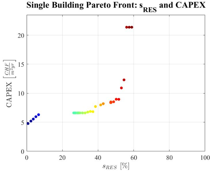
Figure 13: Single building Pareto curve for LV transformer *HÔPITAL-TR3716*
