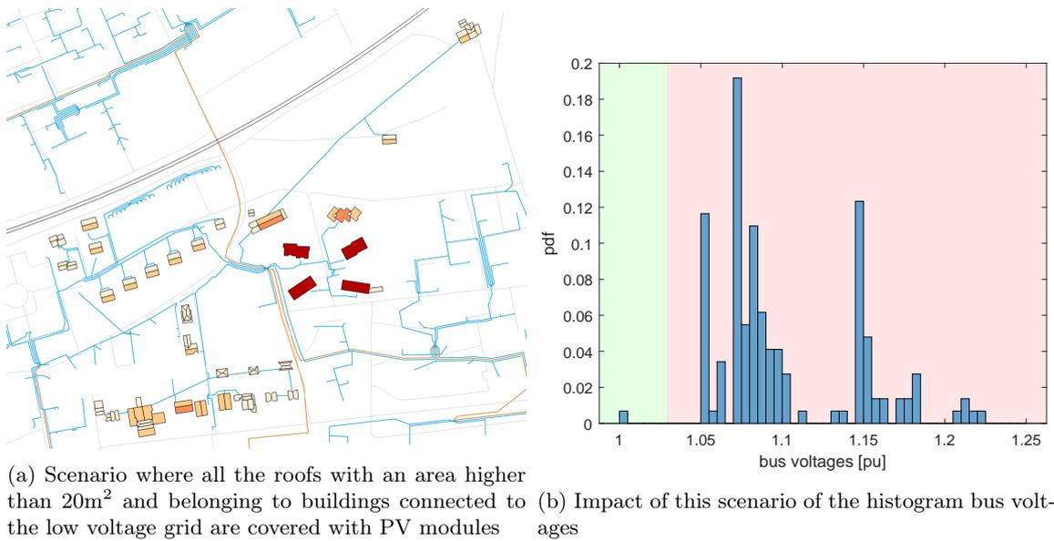
(a) Scenario where all the roofs with an area higher than  $20 \text{ m}^2$  and belonging to buildings connected to the low voltage grid are covered with PV modules (b) Impact of this scenario of the histogram bus voltages
