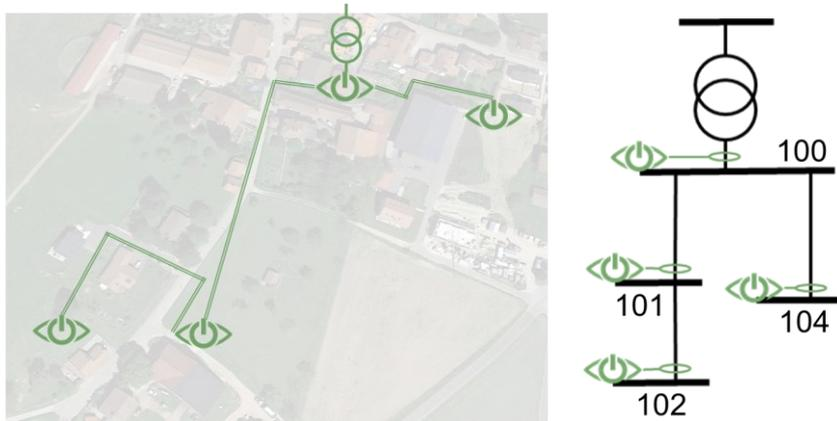
Figure 9. Reduced single line diagram of LV grid of Chapelle-sur-Moudon and location of GridEye devices used for calculation of sensitivity coefficients.
