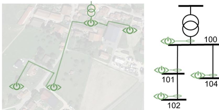
Figure 28. Reduced single line diagram of LV grid of Chapelle-sur-Moudon and location of GridEye devices used for grid analysis.
