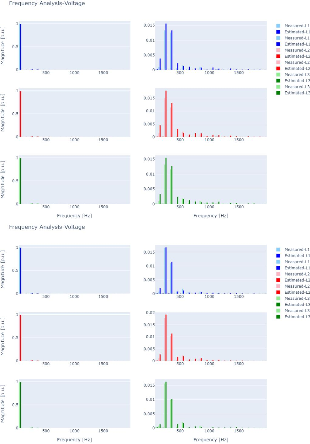
Figure 19. Frequency analysis of the estimated and measured MV voltages; **top)** recorded waveforms in 2017, and **bottom)** recorded waveforms in 2021
