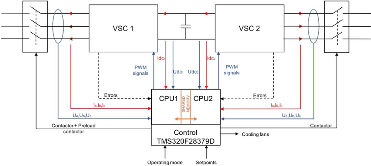
Figure 10: SOP schematics (principle).
