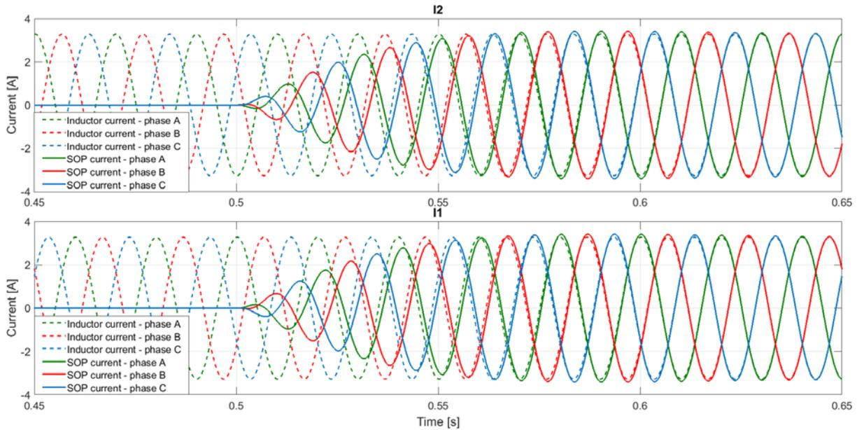
Figure 8: IMPEDANCE mode results,  $L_{ref} = 300 [\mu H]$ .
