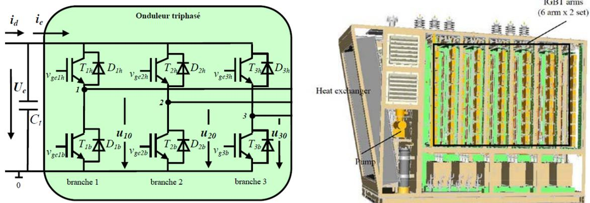
Figure 3- Left picture: 2-level inverter topology; Right picture: SOP using 2-Level inverter [9]
