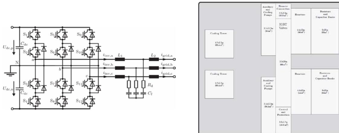
Figure 4-Left picture: 3-level NPC inverter topology; Right picture: Sizing for a 36 MW/15.9 kV back-to-back utility-scale conversion system [12]
