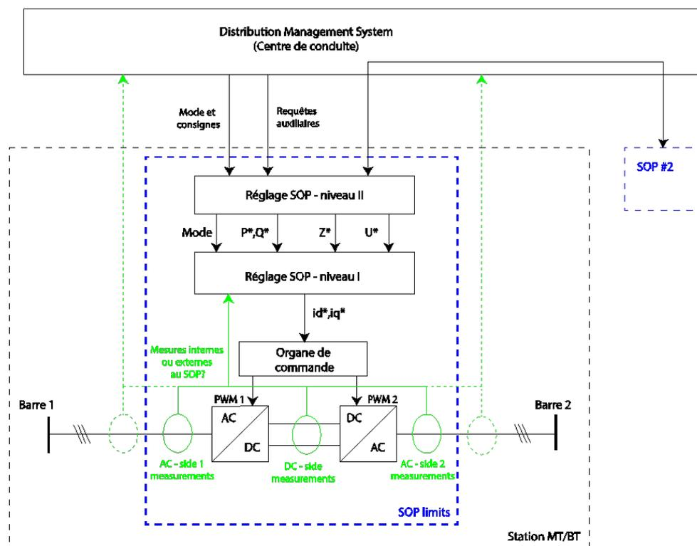
Figure 2: Control architecture of the SOP.
