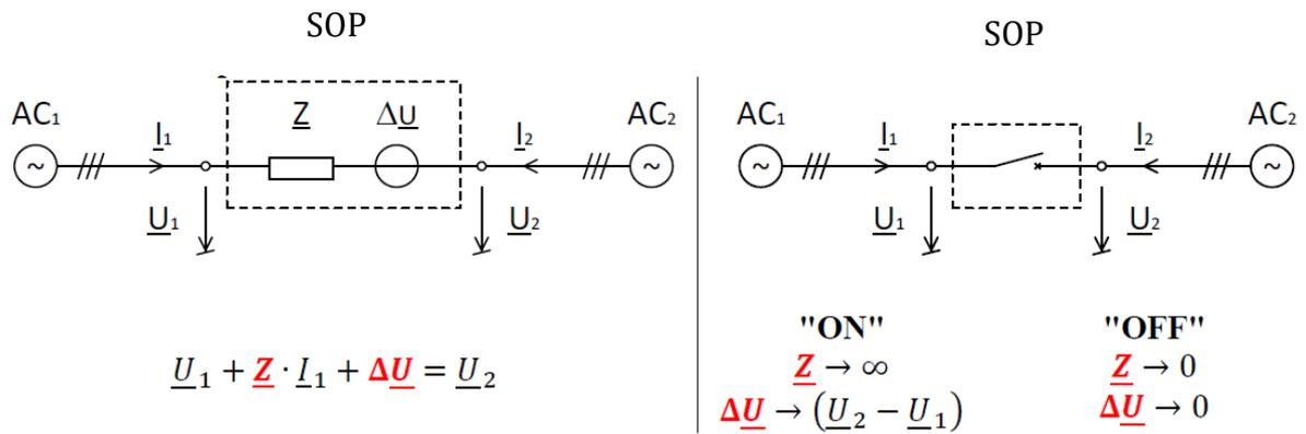
Figure 5: ON/OFF mode principle
