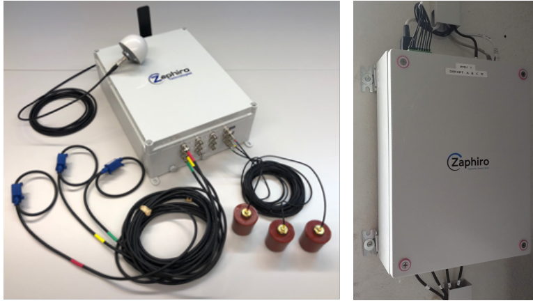
Figure 5: Adopted PMU by Zaphiro Technologies with GPS antenna and current and voltage sensors (left) and installation at the Aigle demonstrator site (right).
