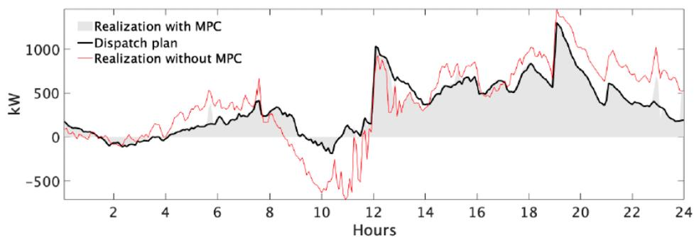
Figure 2. Dispatch plan and slack power with and without the OPF-based MPC BESS control.
