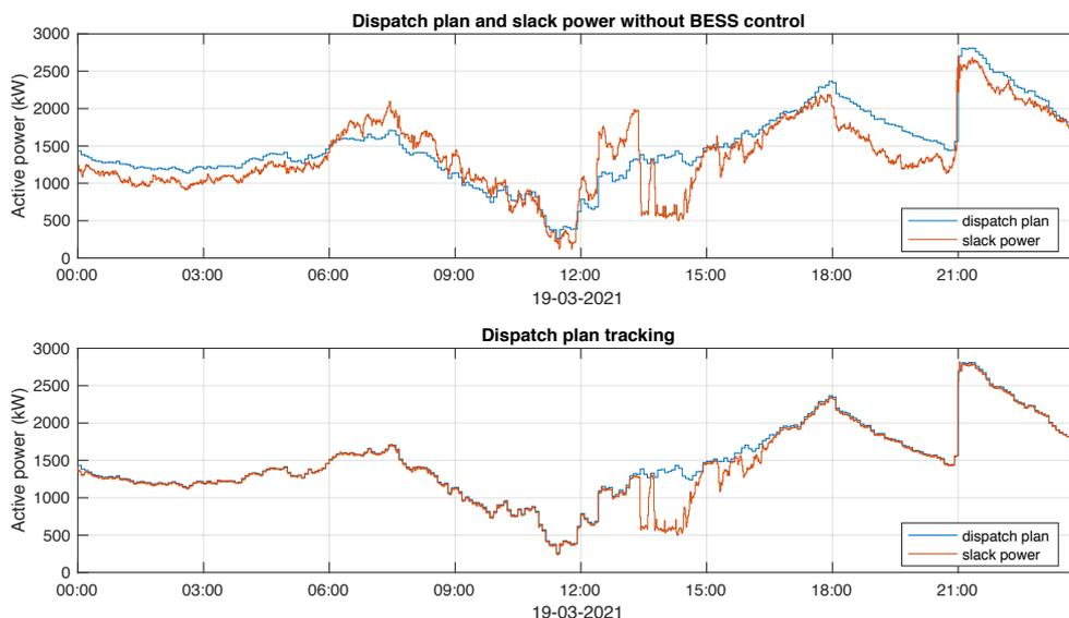
Figure 4. Dispatch plan and slack power without Commelec BESS control (upper plot) and with COMMELEC BESS control (lower plot).
