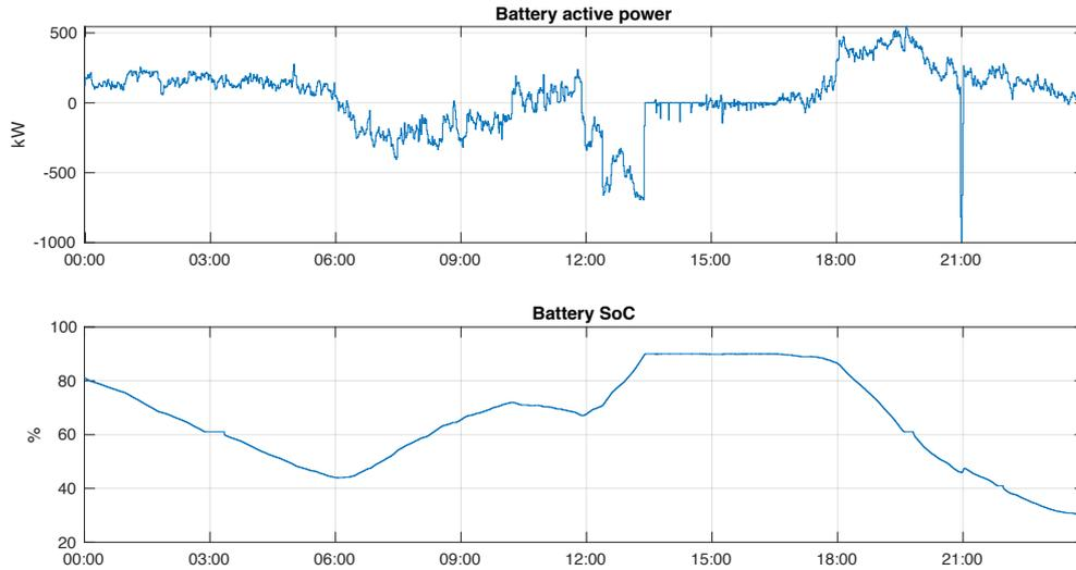
*Figure 5. Measured active power and SoC of the battery in case of COMMELEC control.*
