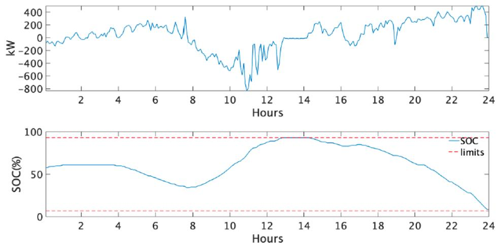
Figure 3. Measured BESS active power for tracking the dispatch plan with the OPF-based MPC BESS control and SoC.
