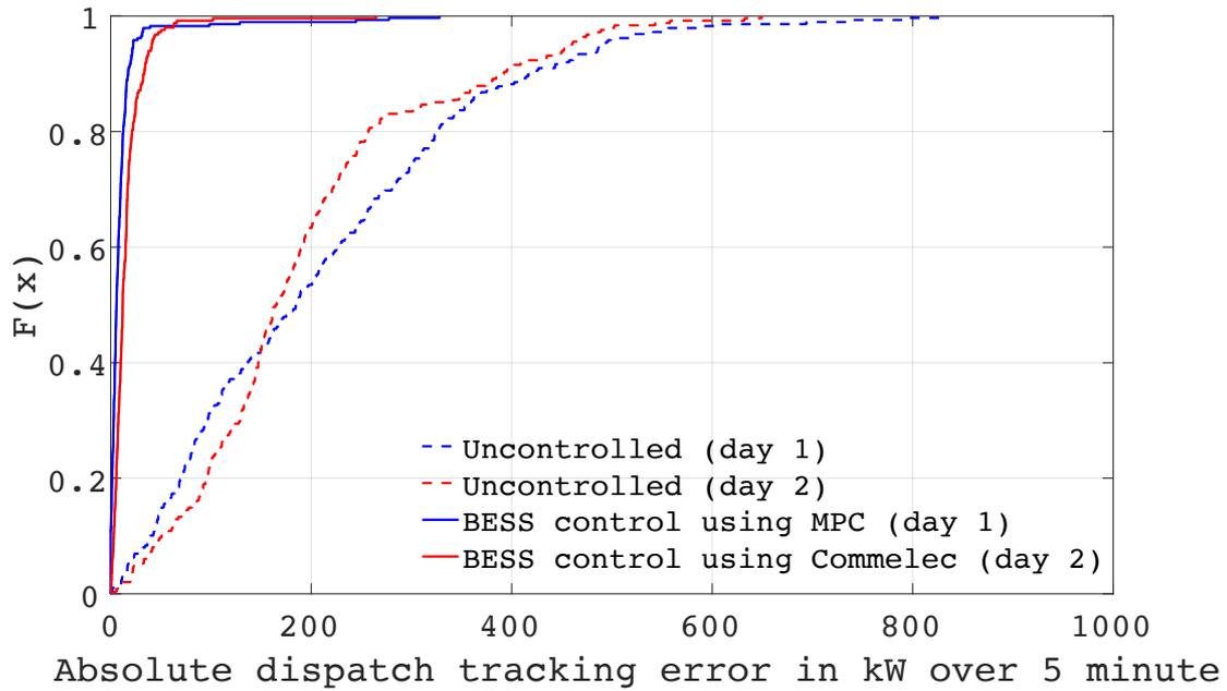
Figure 6. CDF of dispatch tracking absolute difference with and without MPC BESS control (day 1) and with and without COMMELEC BESS control (day 2).
