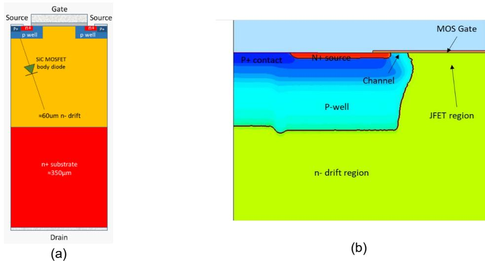
Fig. 12 Schematic cross-section of a 6.5kV MOSFET (a) and TCAD cross-section of the simulated 3.3kV MOSFET active cell (b).
