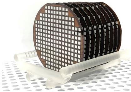
Fig. 1 – SiC MOSFET wafers fabricated from SFOE funded AMPERE project.
