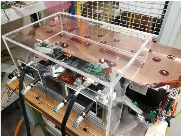
Fig. 24 3.3kV Si IGBT back-to-back monophasic converter.
