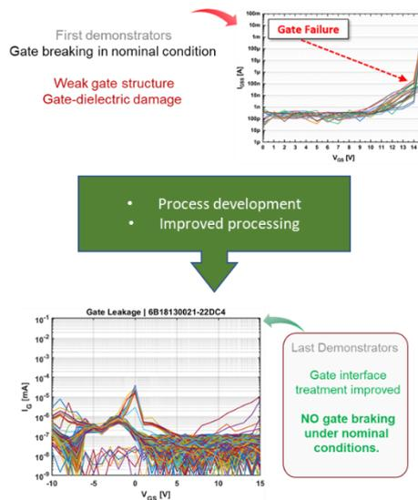
Fig. 8 Evolution of the gate dielectric performance - from the first to the current demonstrators.
