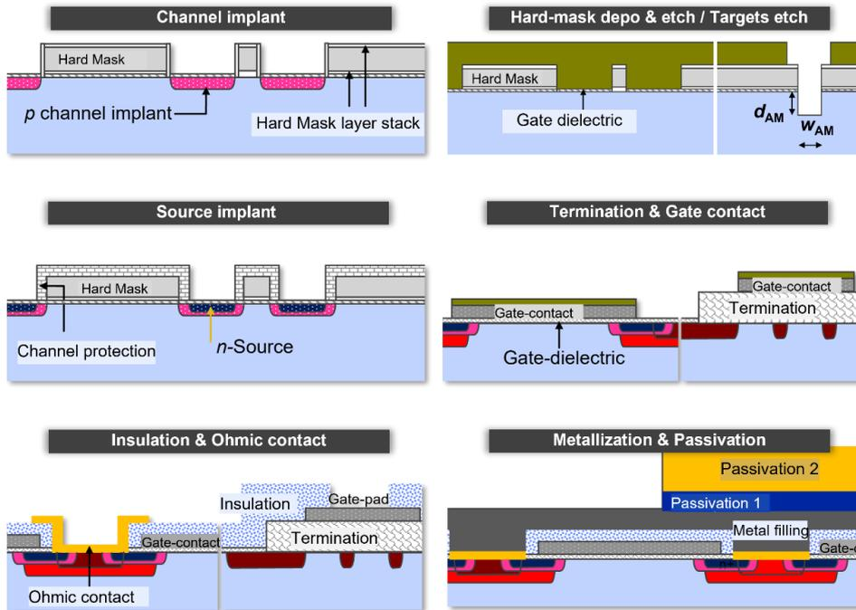
Fig. 6: General overview of most relevant integration steps in the development and manufacturing of SiC MOSFET devices. The different integration steps require several cycles of testing processing conditions and development platforms. The final fabrication router for prototype manufacturing contains about 284 steps.
