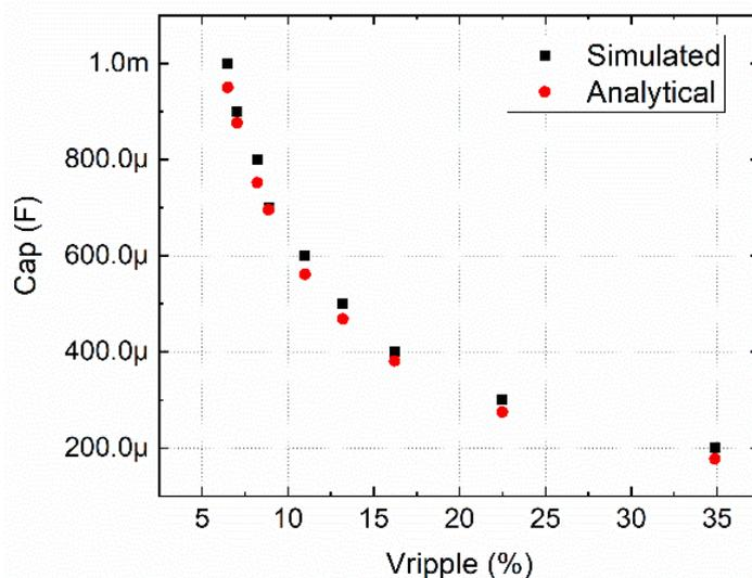
Fig. 20 Capacitance value versus voltage ripple at full load conditions (IL: 300 A, V: 1.8 kV).
