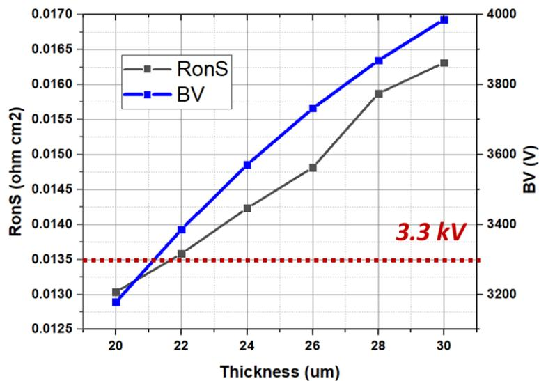
Fig. 10 Ron and VBR dependence on epitaxial layer thickness for a 3.3kV-rated MOSFET.
