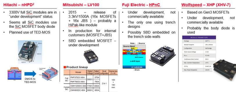
Fig. 4 Summary of 3.3kV full SiC power modules of competitors.
