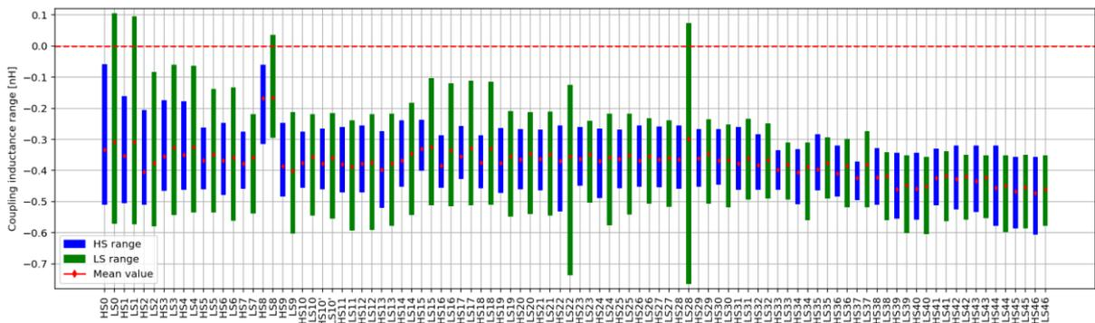
Fig. 15: Coupling inductance ranges of different design iterations for HV SiC LinPak module.
