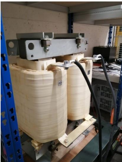
Fig. 22 Monophase load inductor. The inductor weighs 260 kg with dimensions of 485 x 385 x 730 mm.
