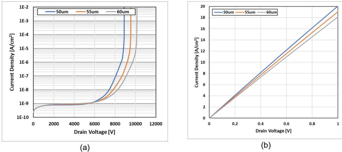
Fig. 13 VBR and Ron dependence on the thickness of the epitaxial layer for a 6.5kV-rated MOSFET.
