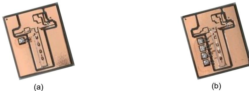
Figure 30: (a) 1x MOSFET and (b) 4x SiC 3.3kV MOSFETs bonded onto LinPak substrates.
