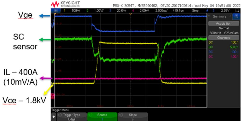
Fig. 40 3.3 kV Si IGBT LinPak switching curves at 1.8 kV/400 A – 25 °C. The gate curve is Vge, the switched current is represented by the inductor current IL, the collector-emitter voltage is represented by Vce. The SC sensor signal is the device current measured by a non-optimized home-made sensor with high-noise.
