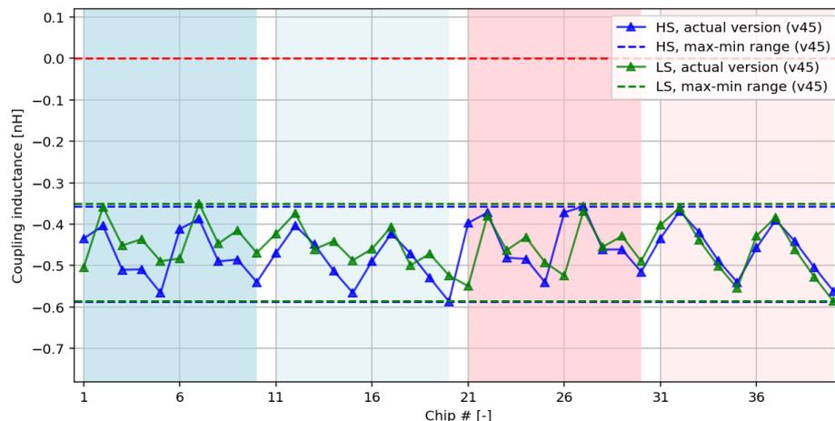
Fig. 16: Coupling inductance values of v45, for HS (blue) and LS (green) switches, per chip.
