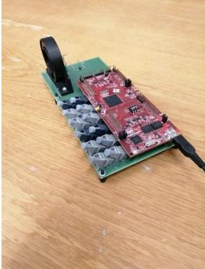
Fig. 23 Microcontroller board with integrated optical connectors and current sensor.
