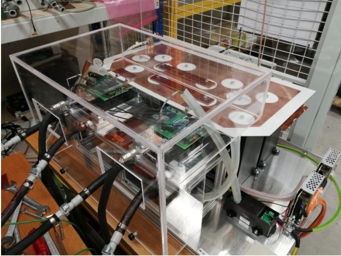
Fig. 26 6.5kV Si IGBT back-to-back monophasic converter.
