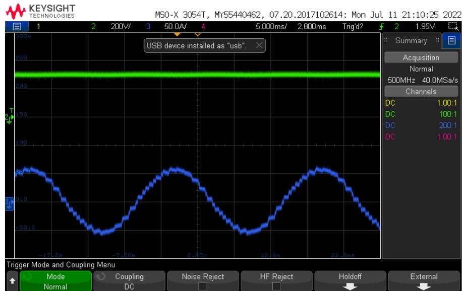
Fig. 42 Inductor load current (sine wave, 50 Hz) and DC link voltage (green - constant DC voltage). Switching frequency of 1 kHz.
