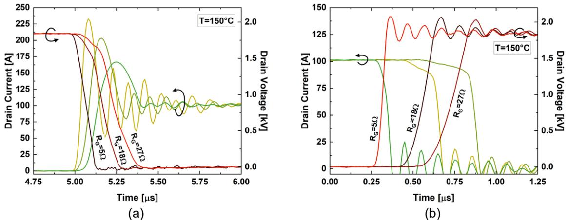
Fig. 32 Turn-on (a) and turn-off (b) waveforms for substrates with 4× devices, at different RG values ( $V_{\text{Nominal}}=1.8\text{kV}$ ,  $I_{\text{Nominal}}=25\text{A/die}$ ,  $V_{\text{GS}}=\pm 15\text{V}$ ,  $T=150^\circ\text{C}$ )
