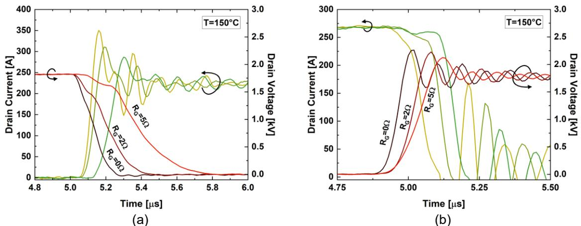
Fig. 36 Turn-on (a) and turn-off (b) waveforms for substrates with 10× devices, for different RG values ( $V_{Nominal}=1.8kV$ ,  $I_{Nominal}=250A$ ,  $V_{GS}=\pm 15V$ ,  $T=150^{\circ}C$ ).
