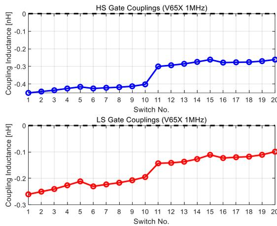
Fig. 17 Coupling inductance values for LV SiC LinPak for 20 chips per side configuration.
