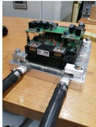
Fig. 21 (Left) Gate driver specifications. (Right) Gatedriver on top of a 3.3 kV Si IGBT Linpack power module with optical connections. The power module is fixed on a cold plate.
