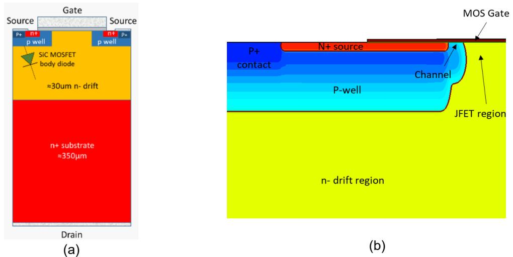
Fig. 9 Schematic cross-section of a 3.3kV MOSFET (a) and TCAD cross-section of the simulated 3.3kV MOSFET active cell (b).
