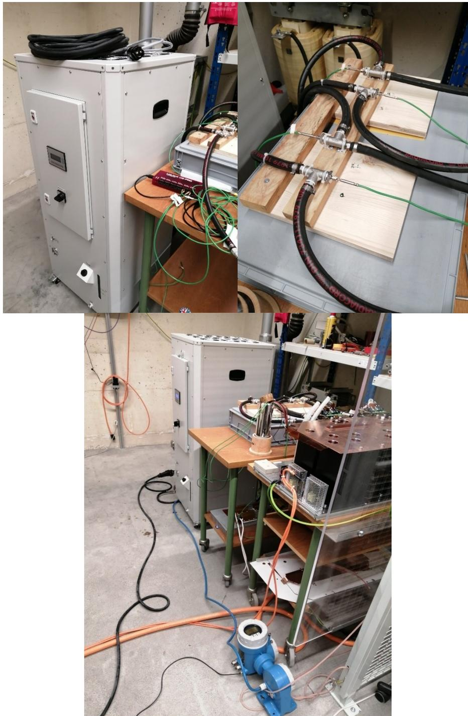
Fig. 27 (Top-left) Chiller unit. (Top-right) Thermocouples placed in the inlet and outlet of each coldplate. (Bottom) Power converter with cooling system.
