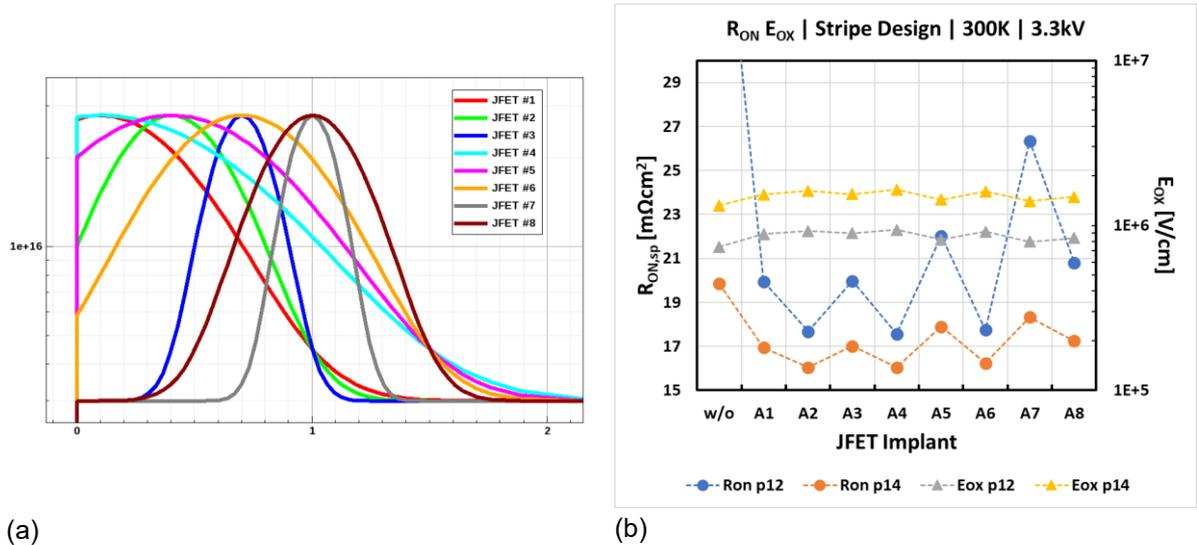
Fig. 11 JFET region profiles investigated (a) and variation of  $R_{on}$  and  $E_{ox}$  with JFET region profile, for 12 and 14 $\mu\text{m}$  cell pitches (b).
