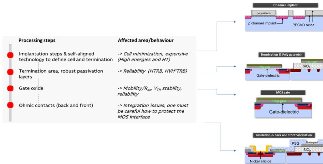
Fig. 7 Schematic chart showing some of the crucial processed needed for the fabrication of a high power SiC MOSFET; schematic cross-sections of a MOSFET during various stages of fabrication are also shown.
