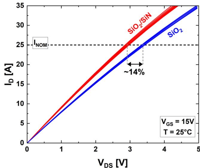
Figure 29: Forward IV of 3.3kV SiC MOSFET using a SiO<sub>2</sub>/SiN as gate dielectric; for reference, IV curves for similarly-rated SiC MOSFETs with SiO<sub>2</sub> gate are also shown.
