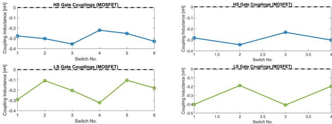
Fig 18 Coupling inductance values for HV Si LinPak, for 3 IGBT+ 2 diode configuration (left) and 2 IGBT + 2 diode configuration (right).
