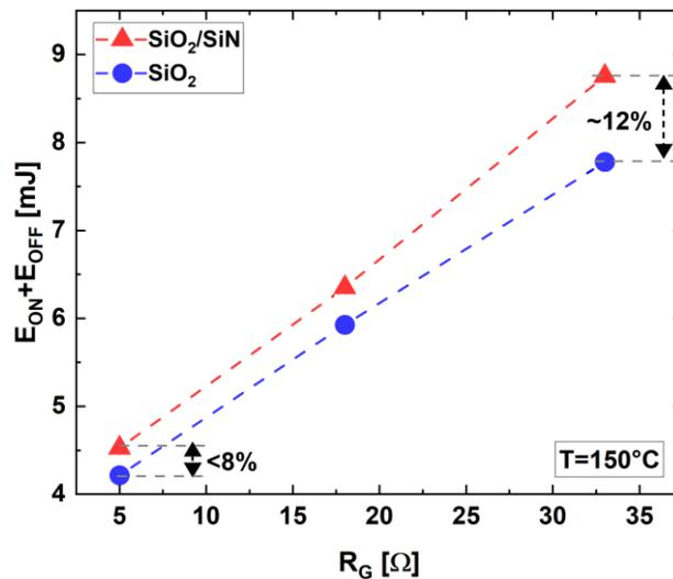
Fig. 34 Comparison of switching energy values for SiO<sub>2</sub> and SiO<sub>2</sub>/SiN stack as gate dielectrics ( $V_N = 1.8\text{kV}$ ,  $I_N = 25\text{A}$ ,  $V_{\text{GS}} = \pm 15\text{V}$ ,  $T = 150^\circ\text{C}$ )
