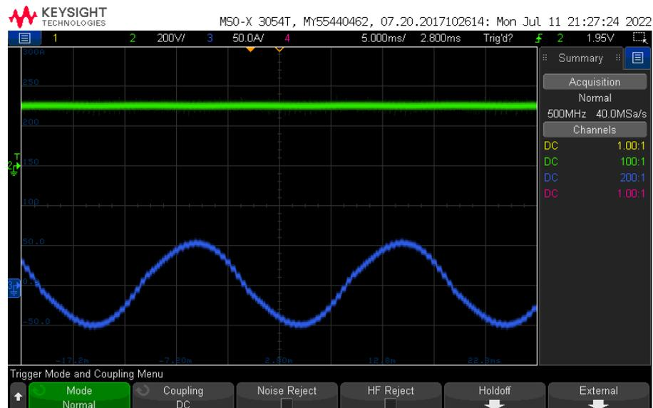
Fig. 43 Inductor load current (sine wave – 50 Hz) and DC link voltage (green – constant DC voltage). Switching frequency of 2 kHz.
