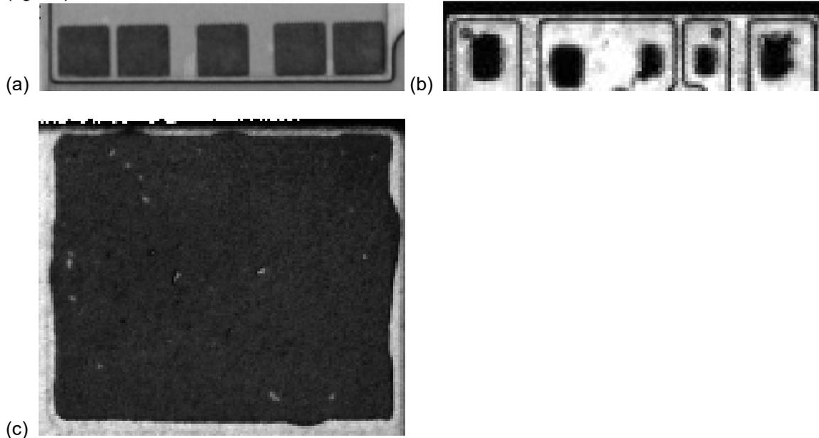
Figure 39. SAM image of (a) sintered chip-substrate attachment, interconnections of 5 chips are shown; (b) ultrasonic welded terminal connection, interconnections of 5 terminal feet are shown; (c) soldered substrate-baseplate connection, 1 substrate is shown.
