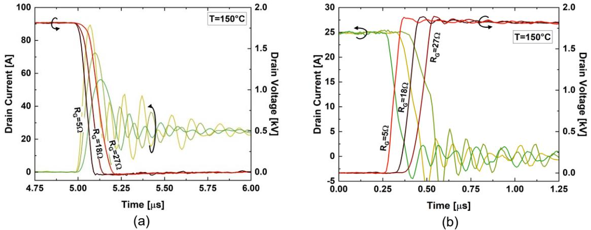
Fig. 31 Turn-on (a) and turn-off (b) waveforms for substrates with 1× devices, at different RG values ( $V_{\text{Nominal}}=1.8\text{kV}$ ,  $I_{\text{Nominal}}=25\text{A/die}$ ,  $V_{\text{GS}}=\pm 15\text{V}$ ,  $T=150^\circ\text{C}$ )
