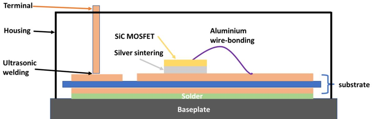
Figure 37: Schematic cross-section of the LinPak demonstrator. The dimensions are not to scale.
