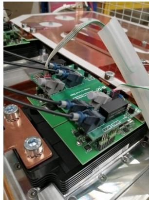
Fig. 25 (Left) Gate driver specifications. Right) Gatedriver on top of a 6.5 kV Si IGBT Linpack power module with optical connections. The power module is fixed on a cold plate.
