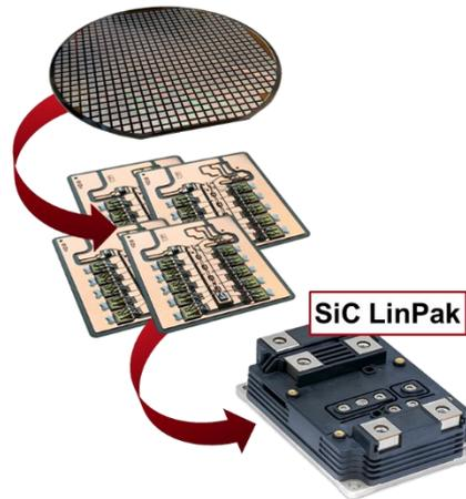
Fig. 35 SiC MOSFETs wafers towards LinPak substrates towards LinPak module chart.
