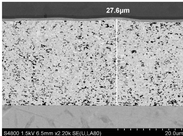
Figure 38. Silver sintering joint. From top to bottom: chip, silver sintering (27.6 μm), substrate.
