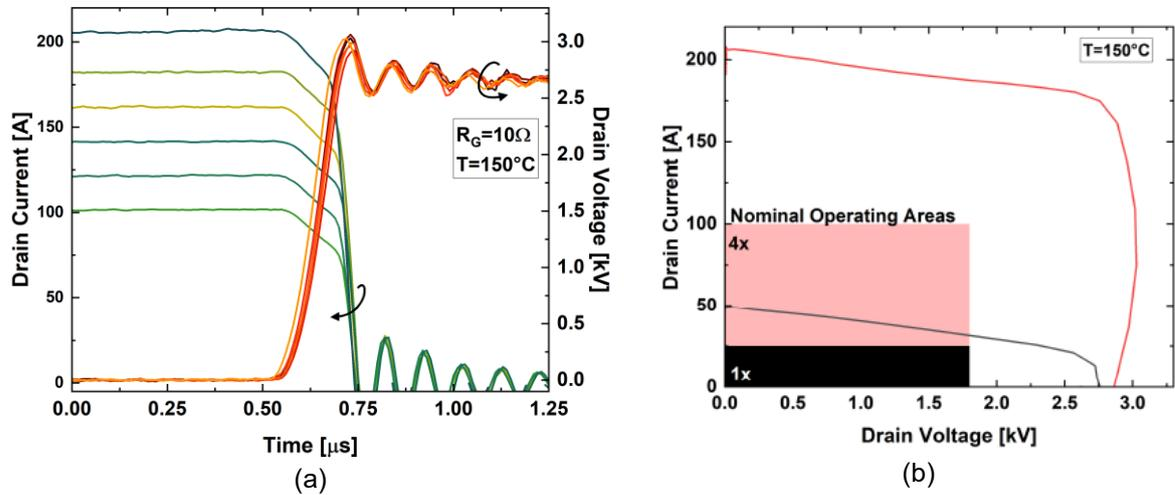
Fig. 33 Turn-off waveforms for substrates 4x devices (a), at different current values; RBSOA extracted from the switching I-V (b) ( $V_{\text{SOA}} = 2.6\text{kV}$ ,  $I_{\text{SOA}} = 50\text{A/die}$ ,  $V_{\text{GS}} = \pm 15\text{V}$ ,  $T = 150^\circ\text{C}$ )
