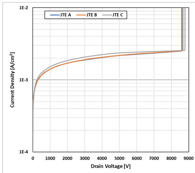
Fig. 14 Blocking curves for a 6.5kV-rated JTE-based edge termination; three different doses have been simulated.
