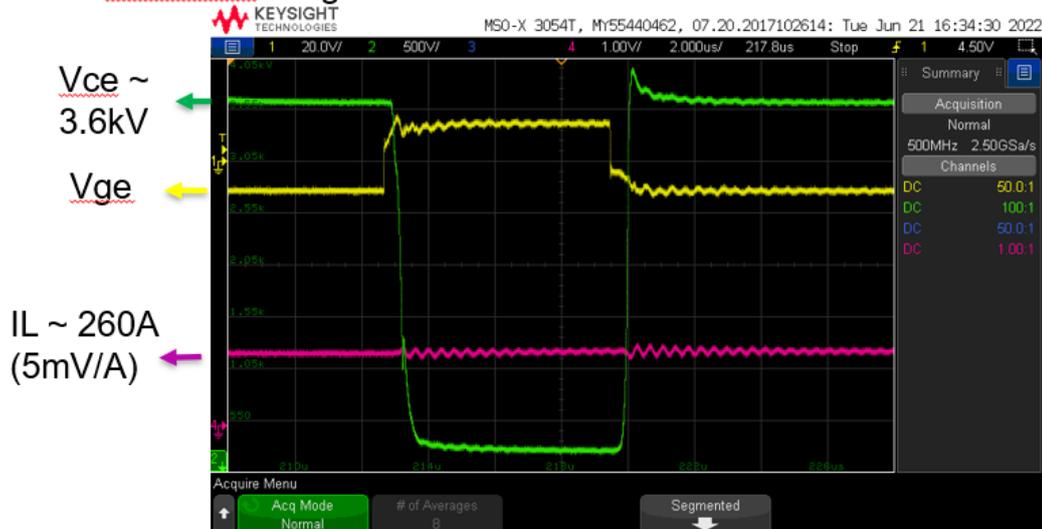
Fig. 41 6.5 kV Si IGBT LinPak switching curves at 3.6 kV/260 A – 25 °C. The gate curve is Vge, the switched current is represented by the inductor current IL, the collector-emitter voltage is represented by Vce.
