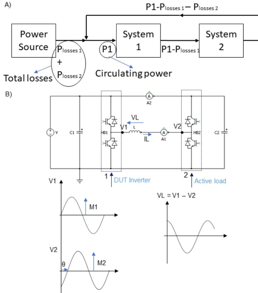
Fig. 19 Single line diagram of Half-bridge converter characterization tester.
