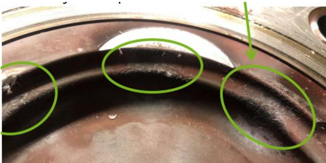
Figure 52: Combustion marks on piston
