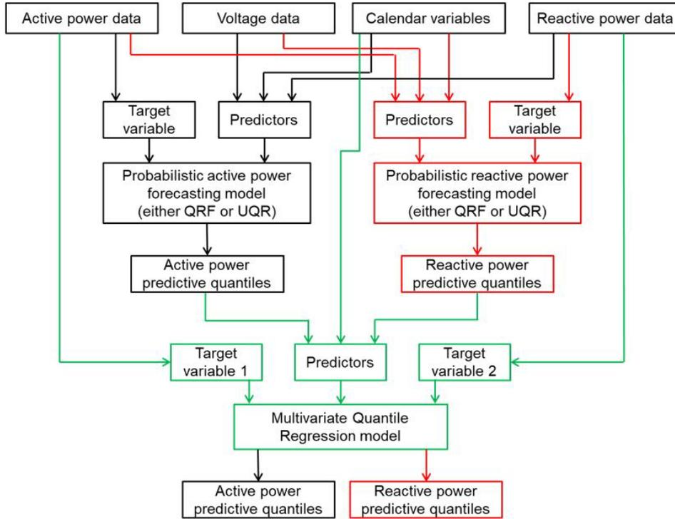
Figure 4: Forecasting methodology for load power consumption based on BBQR approach.
