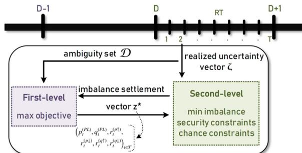
Figure 5: Two-level formulation of the optimization algorithm.
