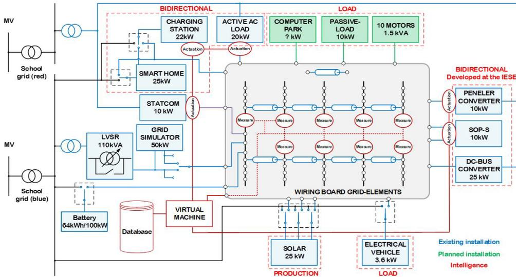
Figure 7: Configuration of Relne laboratory and connected elements.
