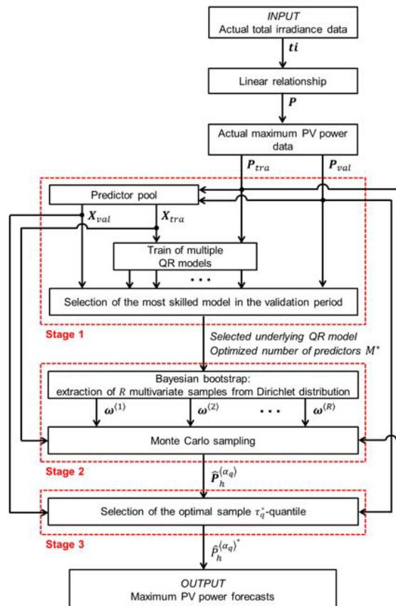
Figure 3: Forecasting methodology for PV power systems based on BBQR approach.
