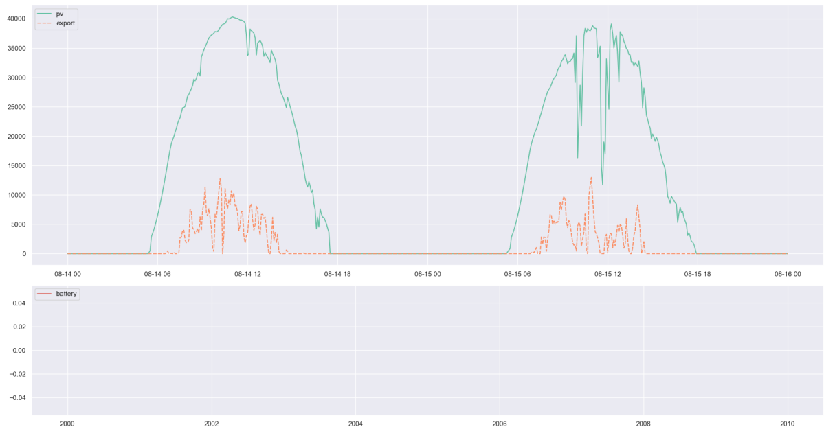
Figure 21: LIC without Battery control detail 14 and 15 August 2021
