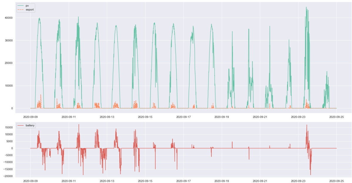
Figure 18: LIC with Battery control, limited power to 20kW, from 9.9.2020 to 25.9.2020, self consumption 98.54%
