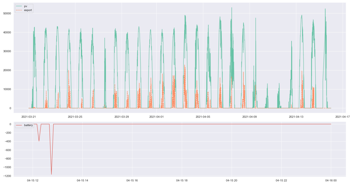
Figure 19: LIC without Battery control from 21.3.2021 to 16.4.2021, self consumption 91.85%
