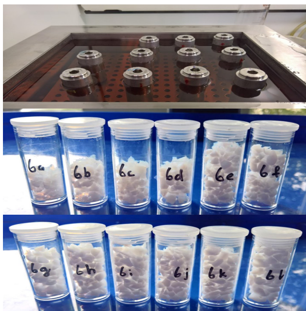
Figure 13: Heating oil bath with lab scaled sample containers (top) and resulting silica aerogel granulate samples.
