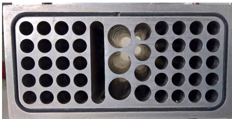
Figure 2: Top view of the 4LR reactor. The different shapes enabled experiments to find the best operating parameters in terms of geometry
