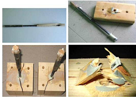
Figure 4.7. Test set-up for investigating the impact of the anchoring length (Johnsson et al. 2007).
