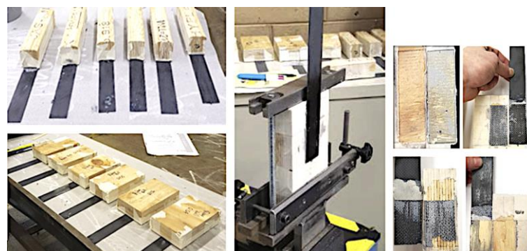
Figure 4.17. Test specimens, test set-up, and failed test specimens. Figure adapted from Subhani et al. (2017b).
