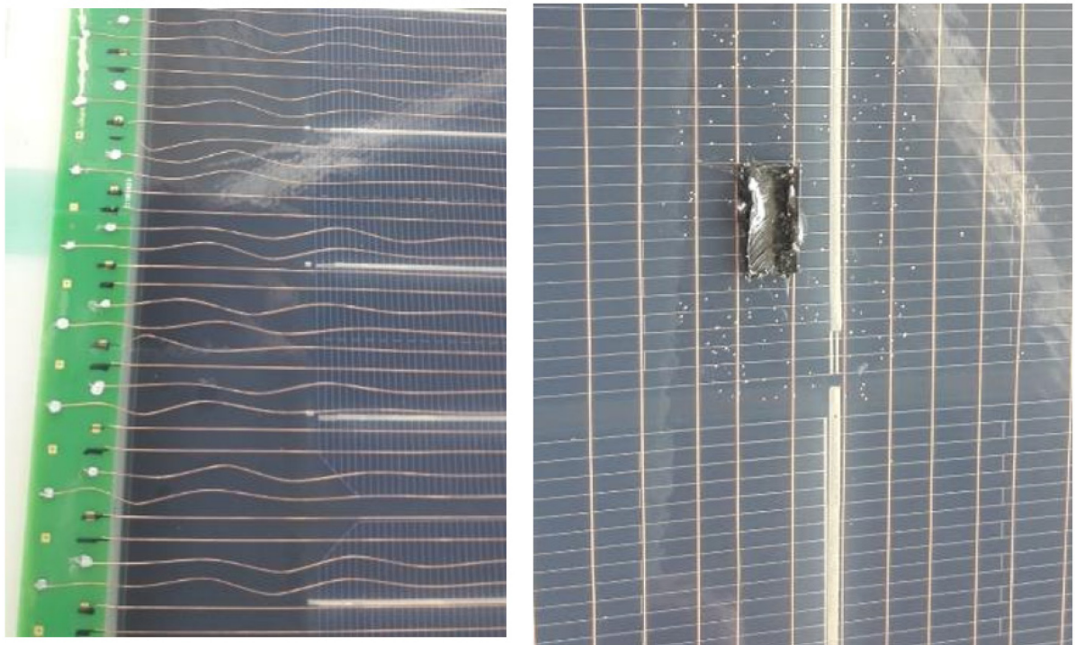
Fig. 4.23 Images of (left) the swimming of the wire due to only one side attachment and (right) repaired shunt between to electrode wire.
