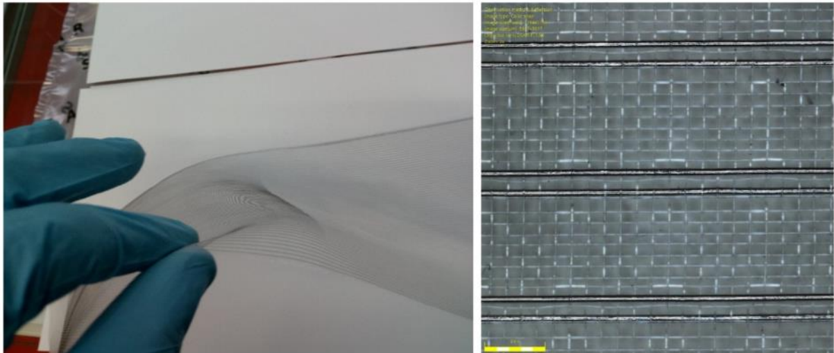
Fig. 3.6. Right: picture of the hybrid mesh from SEFAR and Left: images done with a digital microscope at a magnification of x10, the data-bar is equal to 1 mm.
