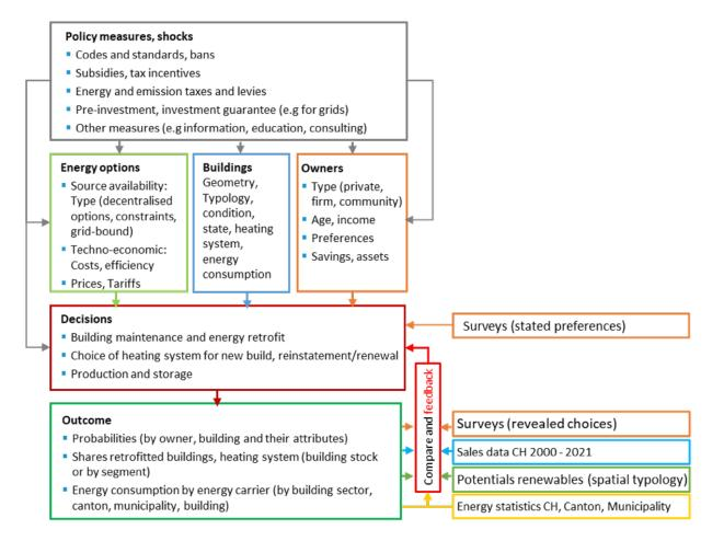
Figure 4: Structure of the sBSM: simplified representation with a focus on the decision module and its calibration.
