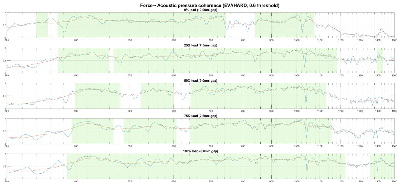
Figure 44 - Force to acoustic pressure coherence for various preloads
