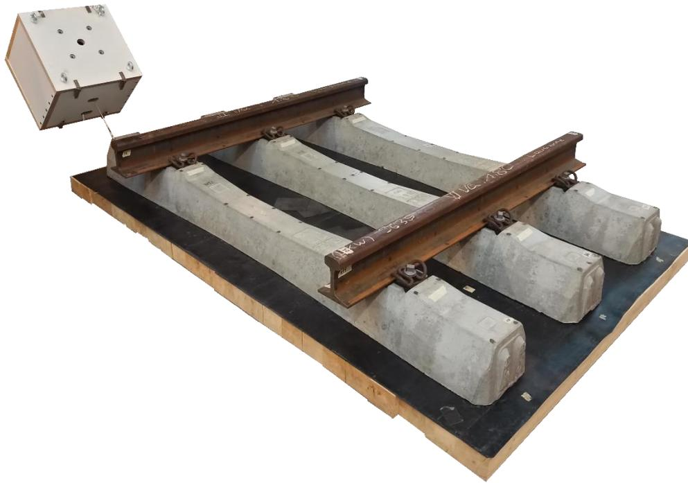
Figure 3 – The three-sleeper unit-cell setup
