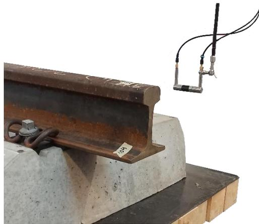
Figure 11 - Pair of microphones for intensimetry measurements
