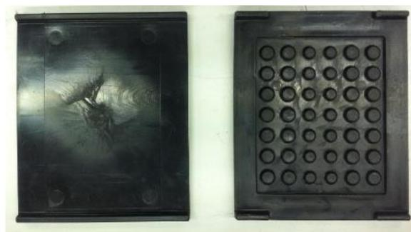
Figure 2 - Hard (left) and soft (right) EVA railpads
