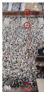
Figure 2.4. a) Installation of the three-sleeper cell at HEIG-VD, showing the shaker (top) and the gantry used for the acoustic measurements. b,c) 12-meter track test set-up used to investigate selected rail pads at TU Munich, showing b) the position of the measurement sensors and c) the shaker.
