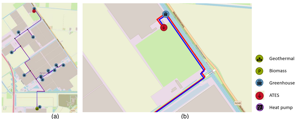
Figure 26: (a) Zoom-out overview ATES location (b) ATES direct coupling to supply green house.
