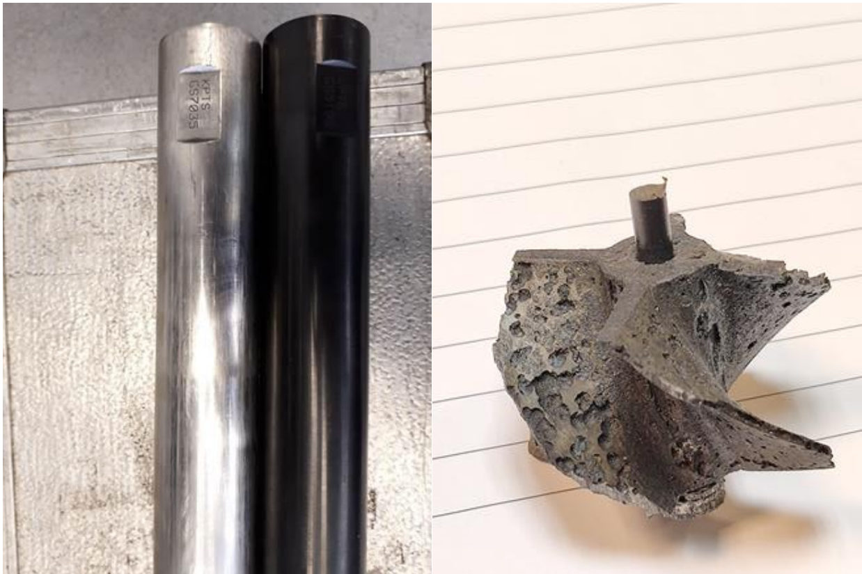
Figure 43: Two examples of the effect of corrosive environment in a superhot geothermal well. Left: A well logging instrument of stainless steel that came black out of a well compared to an instrument of an original color. Right: Corroded spinner from a logging tool.
