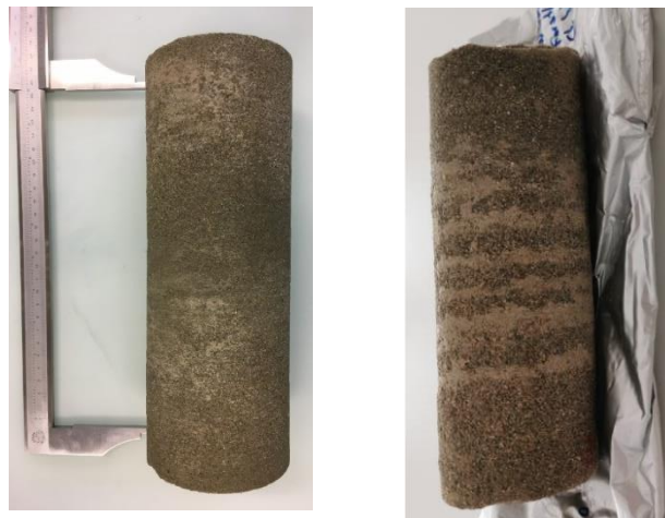
Figure 3.3: USM MB sandstone samples from P7 (sample A on the left, sample B on the right) used for the characterisation of the lithology. Cores are 9.5 cm wide. Both photographs were taken immediately after removing the samples from the hermetically sealed bags and before the samples were fully dry. Therefore, the surface appears relatively dark, especially for sample B.
