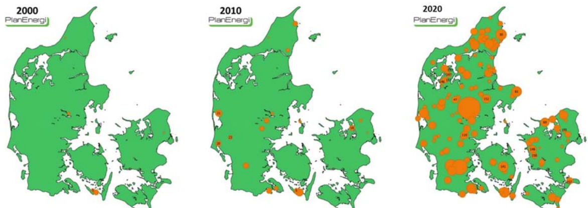
Figure 5.1.1. Evolution of the SDH installations in Denmark between 2000 and 2020 5 . Each circle represents a SDH system and its area is proportional to the surface area of the solar collectors. The figures in the circles show the order in which the SDH systems have been put into operation.
