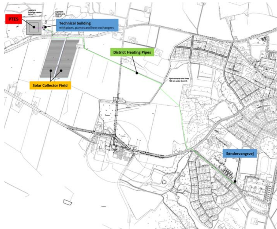
Figure 5.1.5. Location of the solar heating system project and the (green) transmission line to the district heating network of Dronninglund at the boiler plant at Søndervangsvej.
