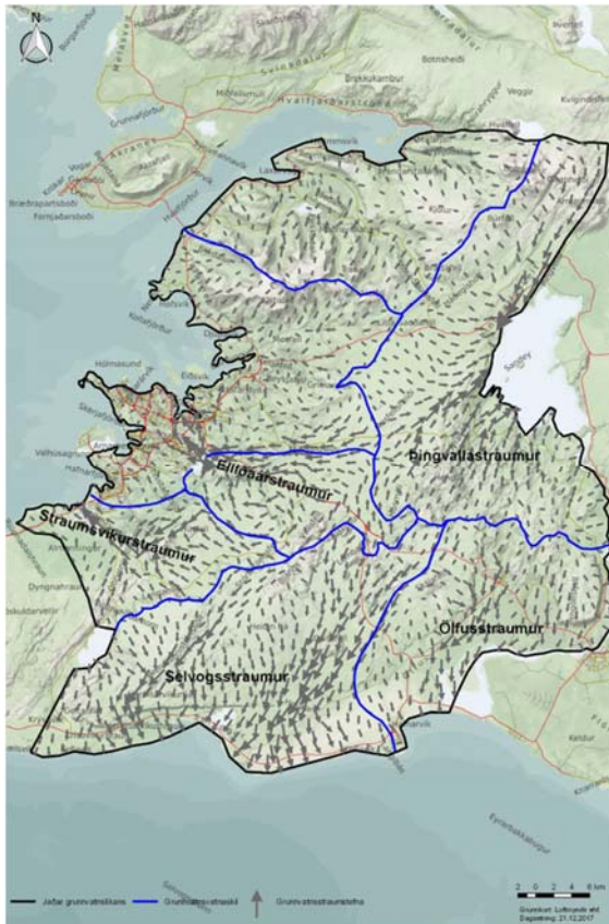
Figure 5.3.5 Calculated shallow groundwater flow in May 1980 when the groundwater divide reached furthest towards the north. The arrows show the direction of the groundwater flow (Vatnaskil, 2017).
