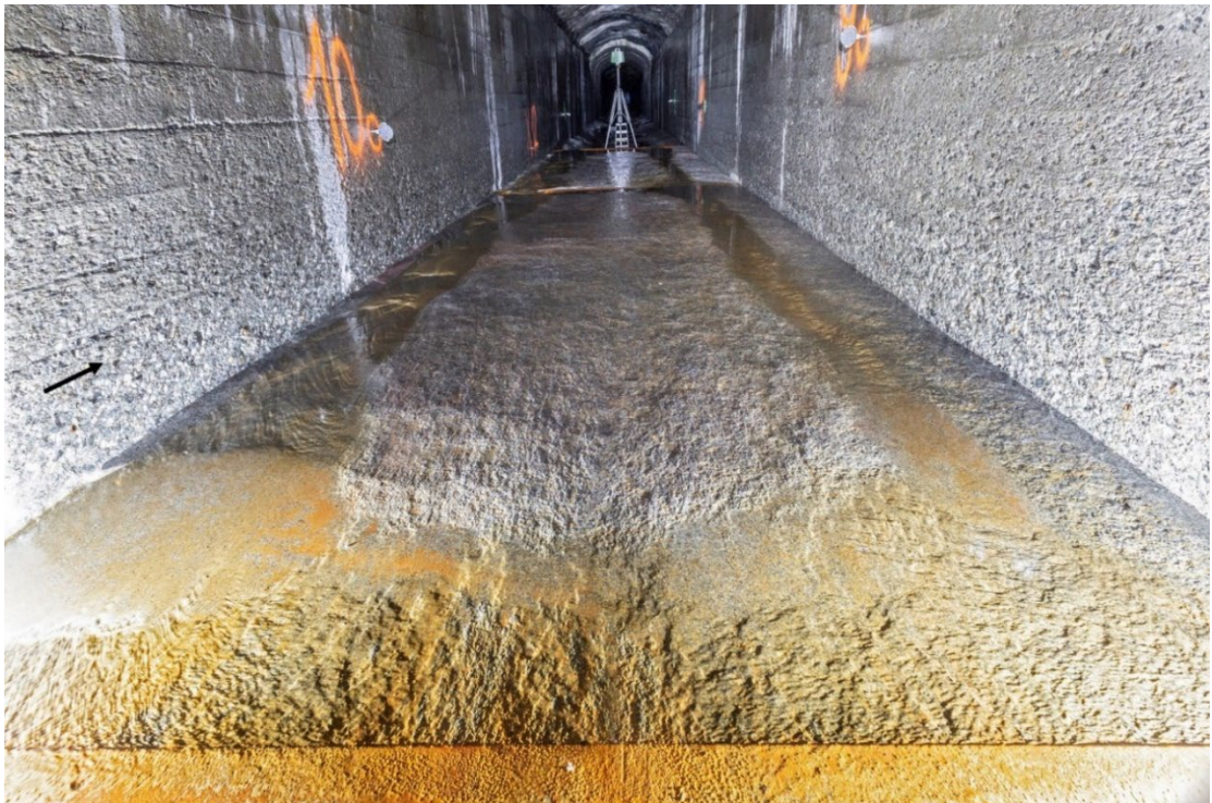
Figure 52: Picture of test field F4 (Steel fiber concrete, SF) during measuring campaign of 4th February 2021 at Runcahez SBT, view in flow direction.
