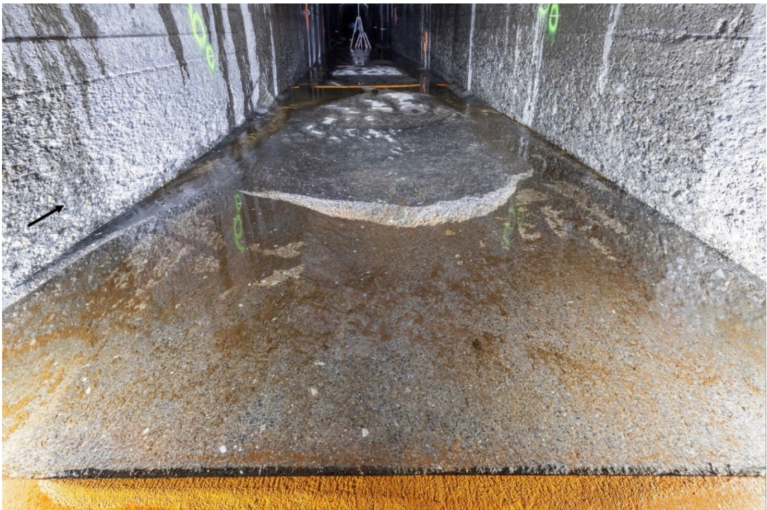
Figure 50: Picture of test field F2 (Roller compacted concrete, RCC) during measuring campaign of 4th February 2021 at Runcahez SBT, view in flow direction.
