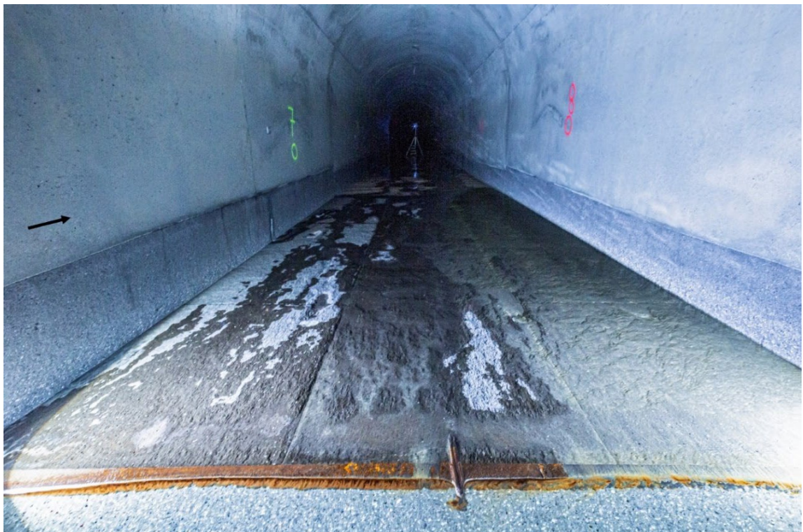
Figure 27: Picture of test field F3 (HAC) during measuring campaign of 10th December 2020 at Solis SBT, view in flow direction.
