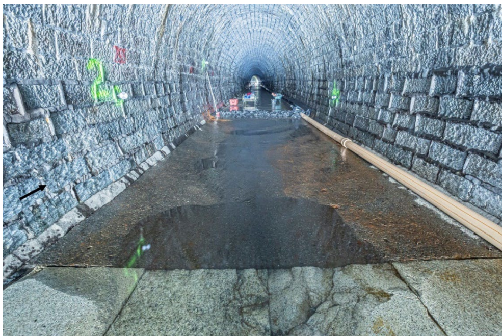
Figure 38: Picture of test field F1 (Concretem C) during measuring campaign of 7th January 2021 at Pfaffensprung SBT, view against flow direction. The local abrasion at the test field transition is not considered.
