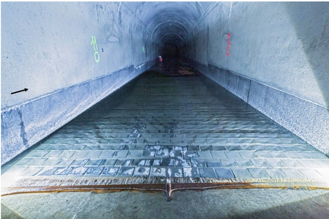
Figure 29: Picture of test field F5 (CB) during measuring campaign of 10th December 2020 at Solis SBT, view in flow direction.
