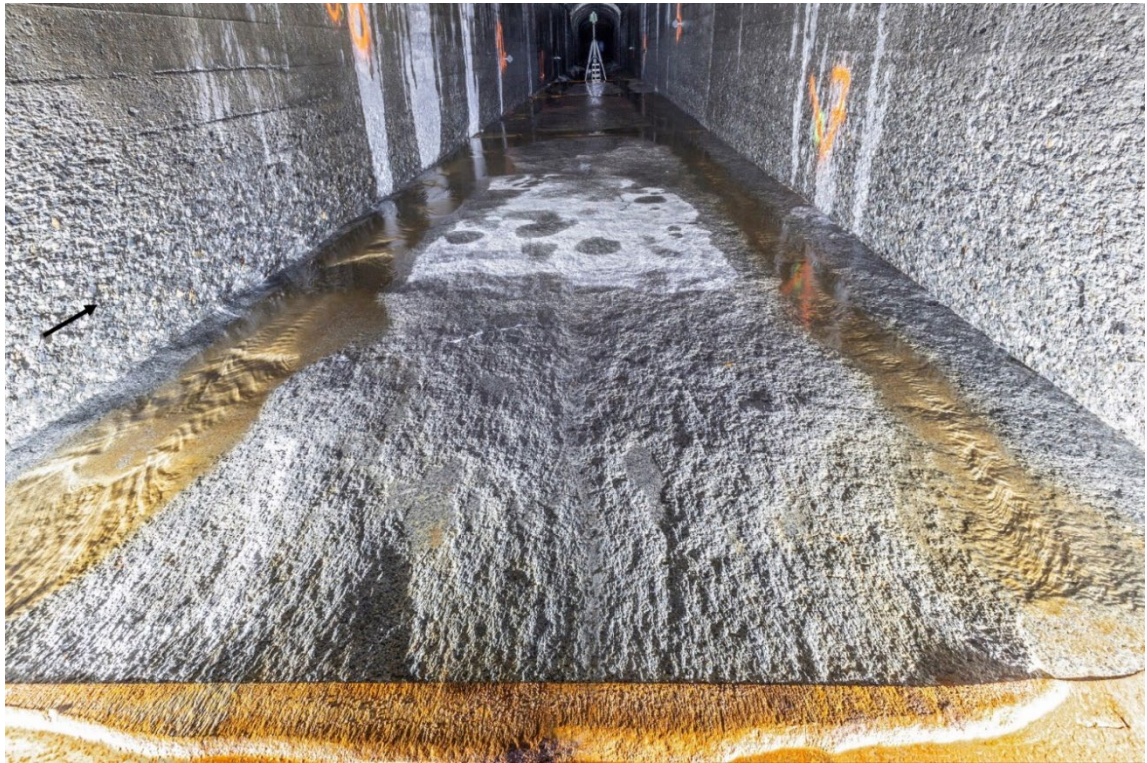
Figure 51: Picture of test field F3 (High performance concrete, HPC) during measuring campaign of 4th February 2021 at Runcahez SBT, view in flow direction.
