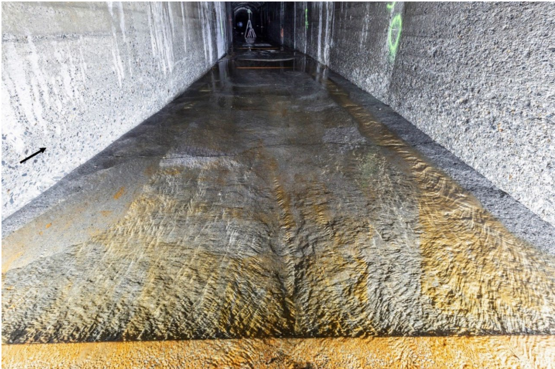
Figure 49: Picture of test field F1 (Silica fume concrete, SC) during measuring campaign of 4th February 2021 at Runcahez SBT, view in flow direction.
